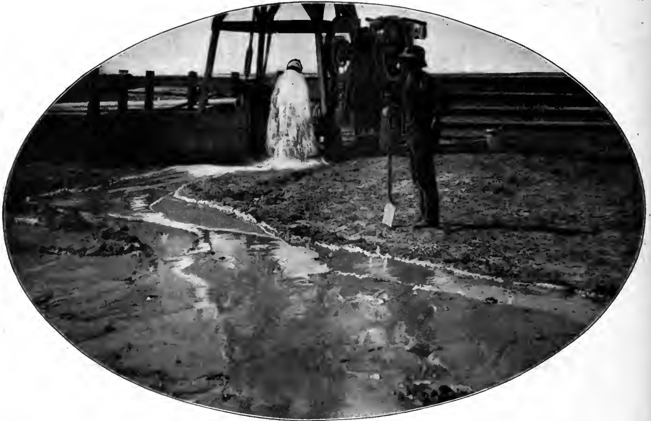
CENTRIFUGAL PUMP AND GASOLINE ENGINE IRRIGATION OUTFIT.
