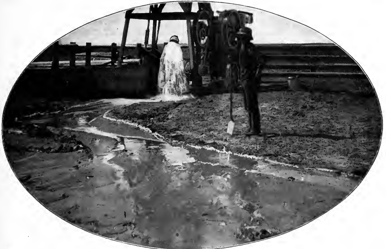
CENTRIFUGAL PUMP AND GASOLINE ENGINE IRRIGATION OUTFIT.
