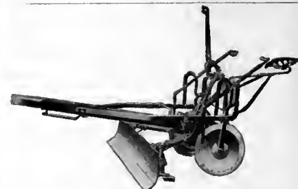
No. 3—MACHINE SET FOR LEVELING.
