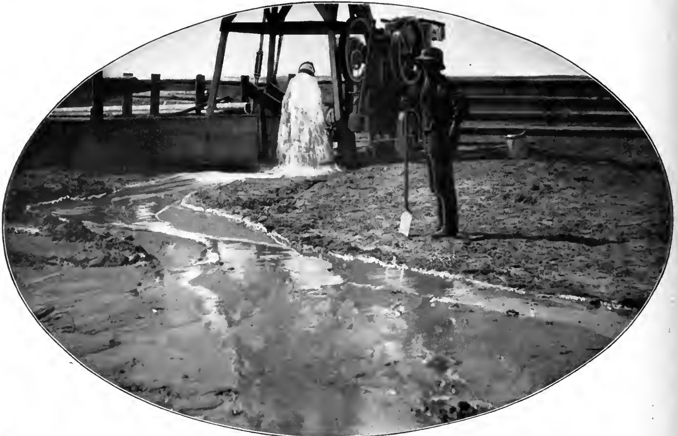
CENTRIFUGAL PUMP AND GASOLINE ENGINE IRRIGATION OUTFIT.
