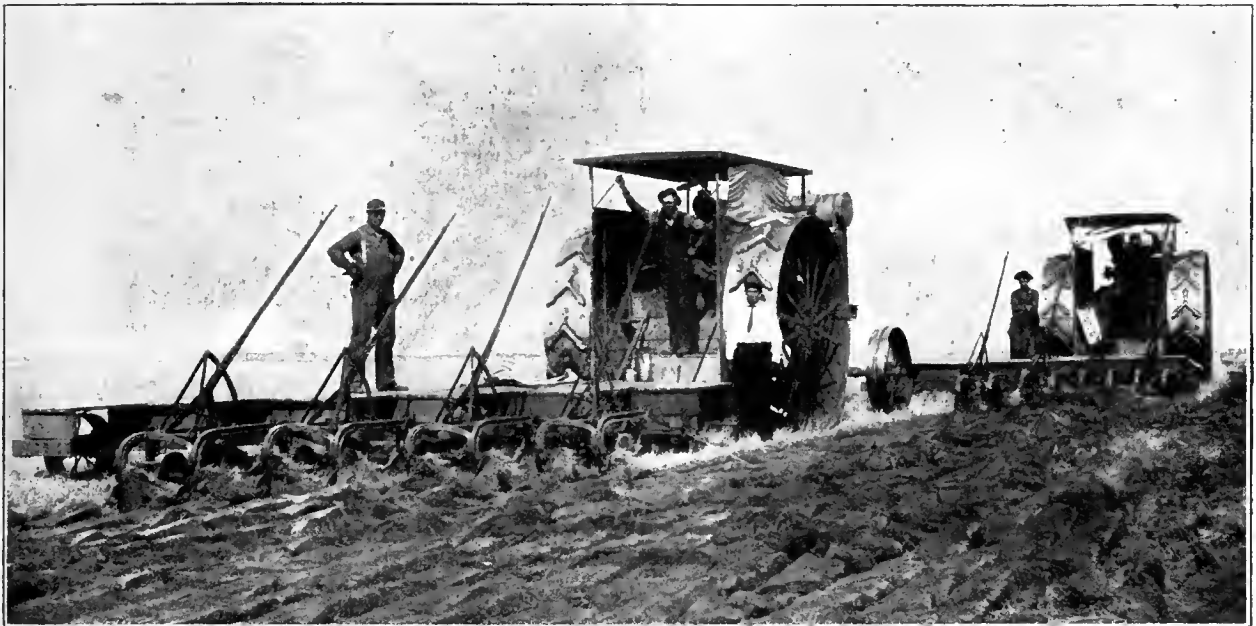
This illustration shows two Flour City Tractors manufactured by Kinnard-Haines Company of Minneapolis, Minnesota. These outfits are owned and operated by Wakefield Bros., at Mott, North Dakota. They are hauling two gangs of 8-14-inch breaker bottoms and have a capacity in raw sod of from 20 to 30 acres per day each. See advertisement on page 456.
