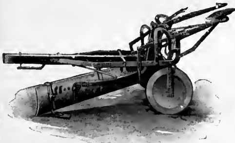
Notice Grader has only two wheels. Both behind blade.
