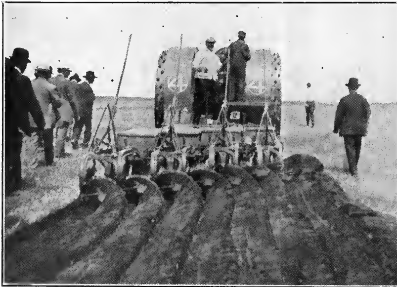
THE BIG FOUR "30" winning the Gold and Silver Medals at Winnipeg, 1911, pulling eight breaker bottoms in tough prairie sod on two gallons of fuel to the acre and making a perfect non-stop run
