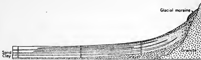
FIGURE 4.—Diagram to illustrate the structure of the artesian basin and the alluvial slope and to indicate the relation of the glacial moraines to the slope.
