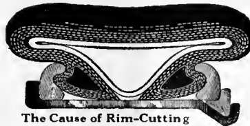
The Cause of Rim-Cutting
