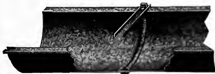
Section of Flume
