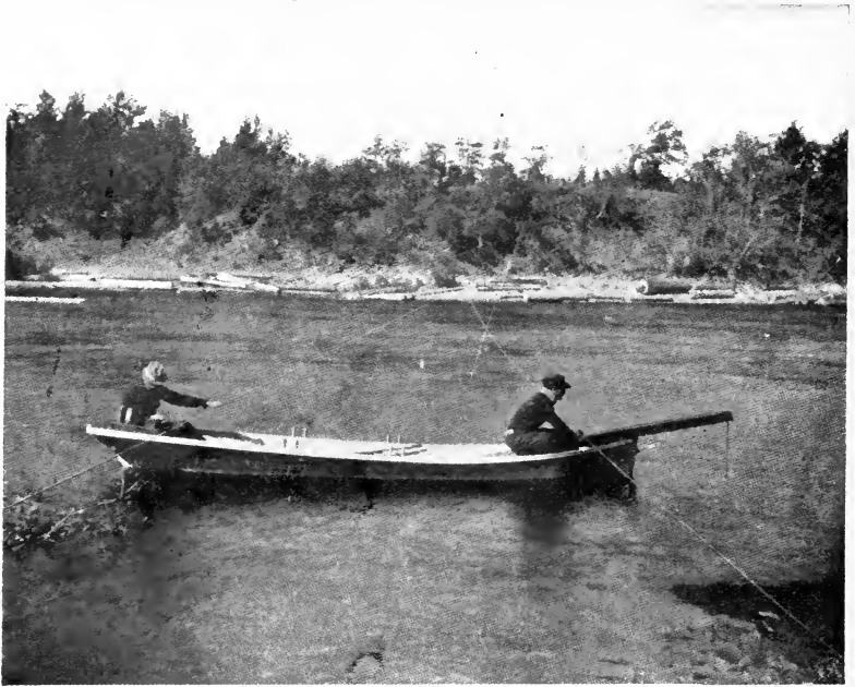
FIG. 53.—Wire and Boat Gaging Station.
