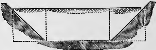
Fig. 129.—PLAN OF MEASURING A CROSS-SECTION.
