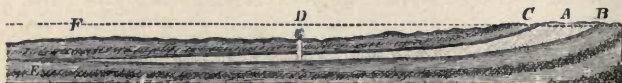
FIG. 78.—Section illustrating the thinning out of a porous water-bearing bed, A , enclosed between impervious beds, B and C , thus furnishing the necessary conditions for an artesian well, D .
