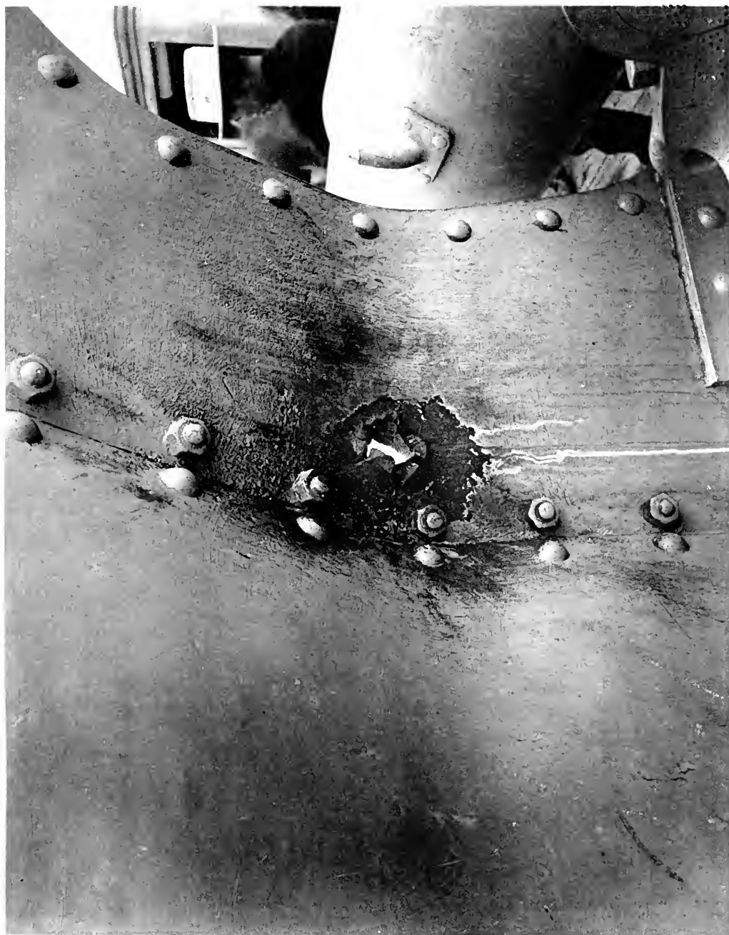
THE "AKAGI" AFTER THE BATTLE, SHOWING THE EFFECT OF A SHIELD ON THE SHIELD OF THE FOURTH GUN.
