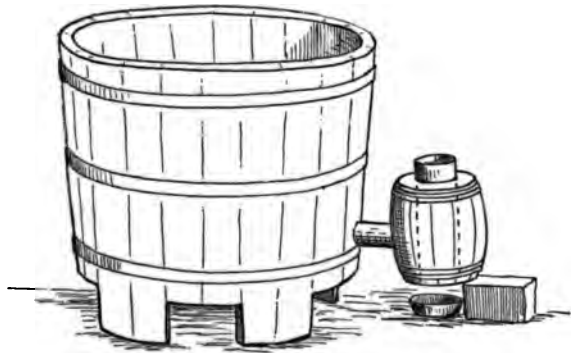
FIG. 183. — BATH-TUB WITH OUTSIDE HEATING-CHAMBER.
