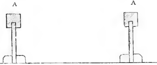
FIG. 22.—SECTION OF BOX OR PIT OF THEATRE. The tops of the partitions (A A) form the Aisles.
