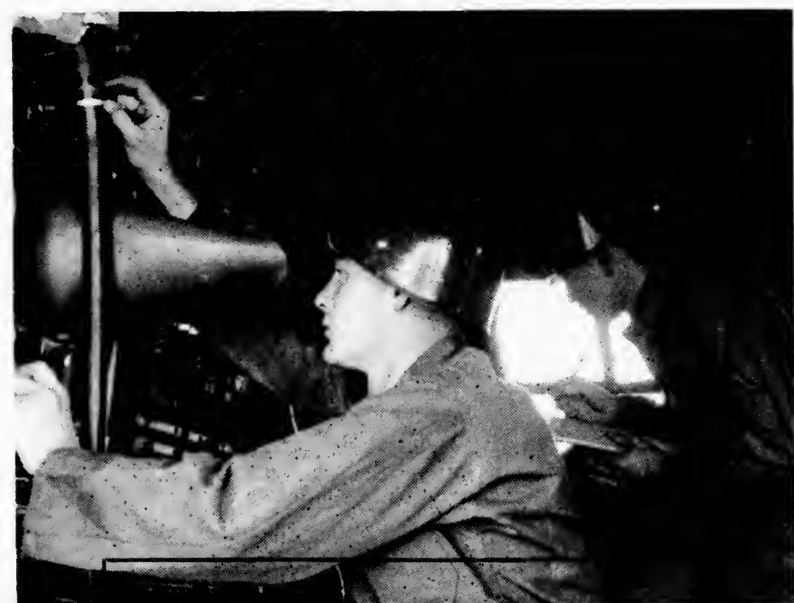
Targets are checked on the position indicator scope of the radar setup
