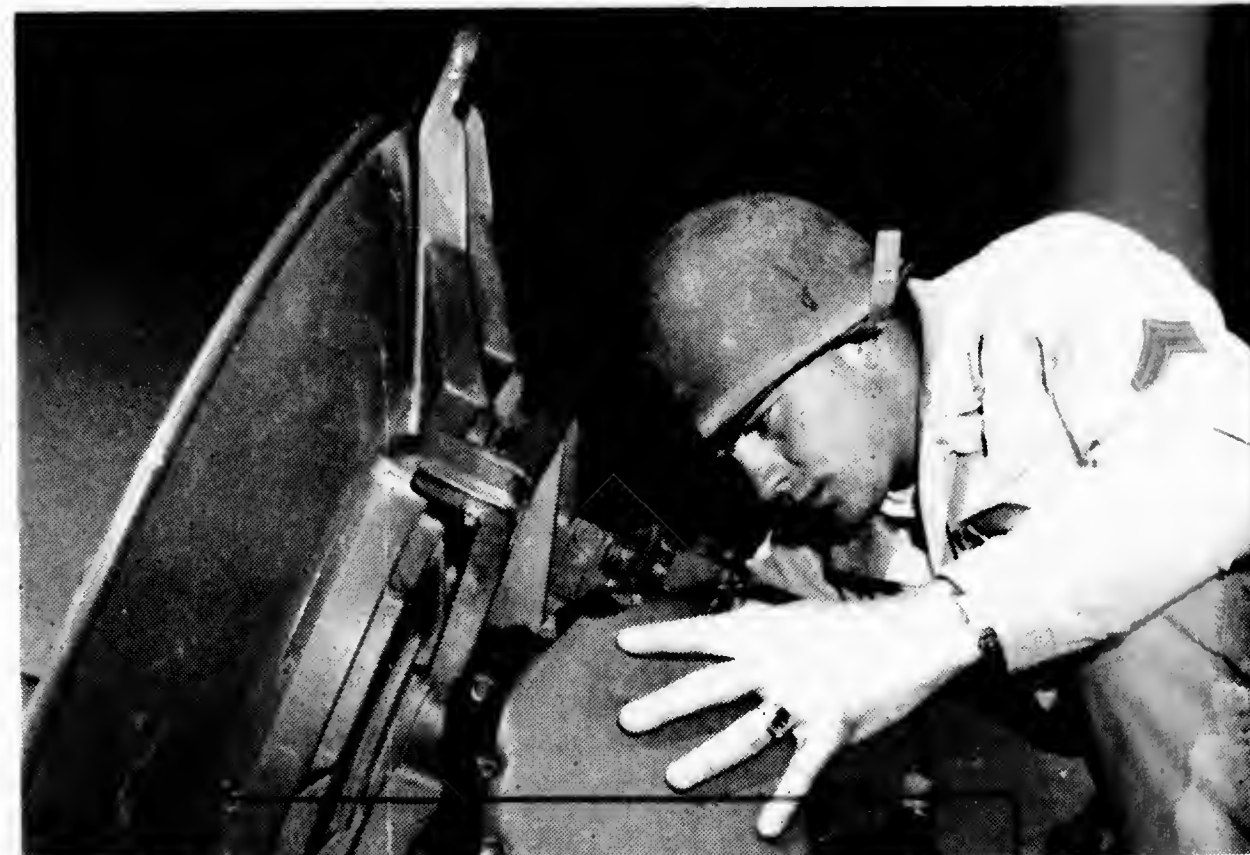
A corporal technician adjusts sensitive parts of the Skysweeper's radar set
