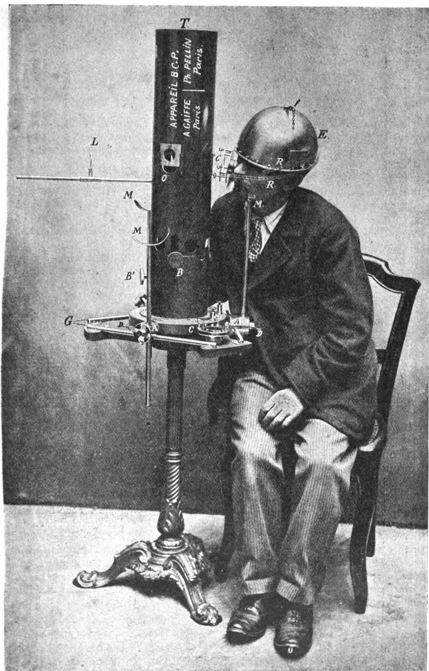
L , Lens throwing upon the wall real and reversed images of cone of light; B , adjustment for the carbons; B' , adjustment of carbons to orifice O ; O , opening for the exit of the rays, with one of the obturators; G , compressor; E , helmet; F , adjustment of air-cushion on inside of helmet; R , steel supports for fixing the compressor to the helmet; A , support for knee-piece; D , screw to regulate the lateral and vertical movements of the chin support M ; G , gliders upon which A moves; T , chimney.
