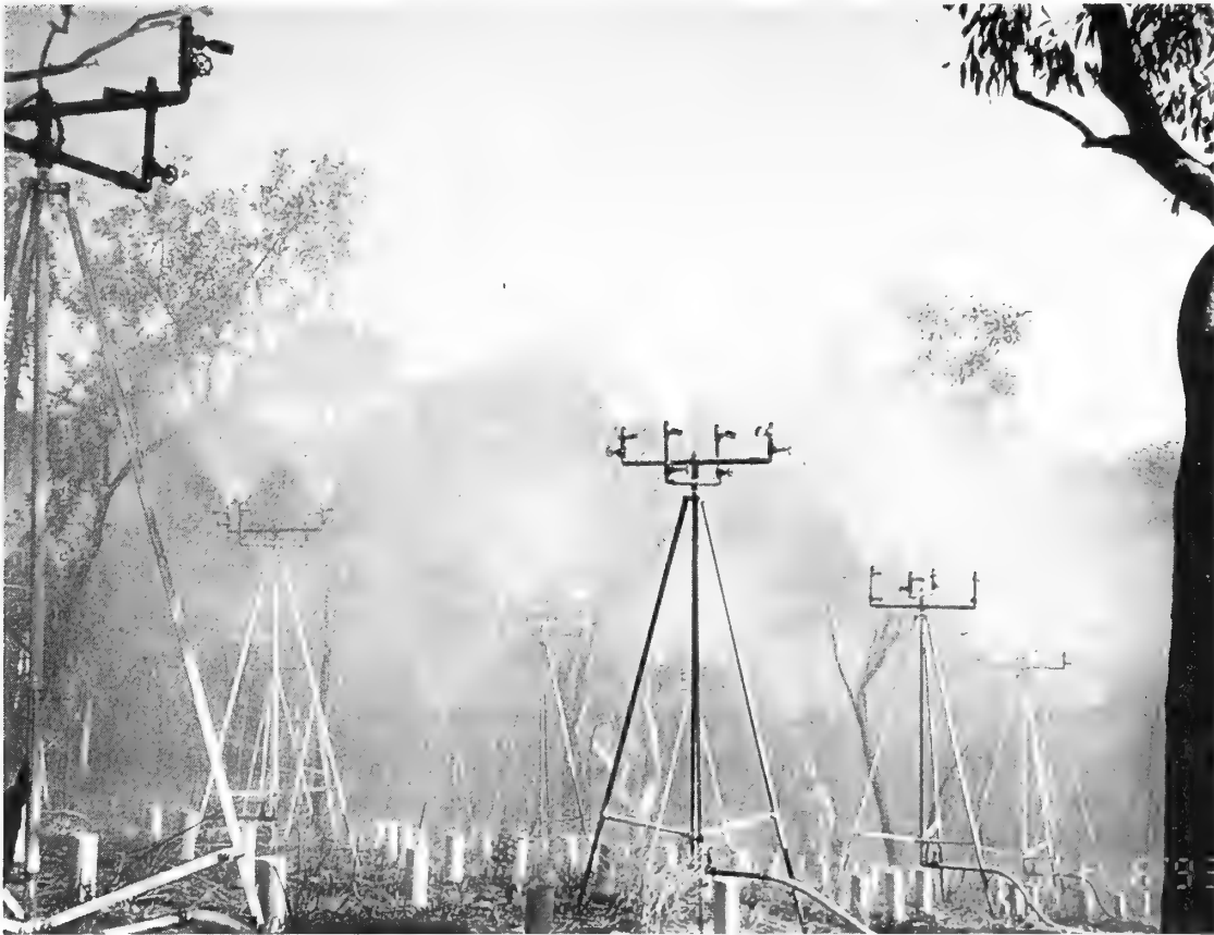
Figure 3a. A rainfall simulation experiment, in which the processes of interrill erosion are studied by monitoring the water and sediment discharge and hydraulic conditions of runoff under specified rainfall intensities.
