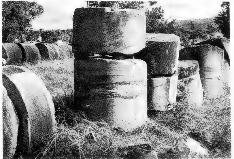
Figure 10. Calyx cores, Warragamba Dam.
