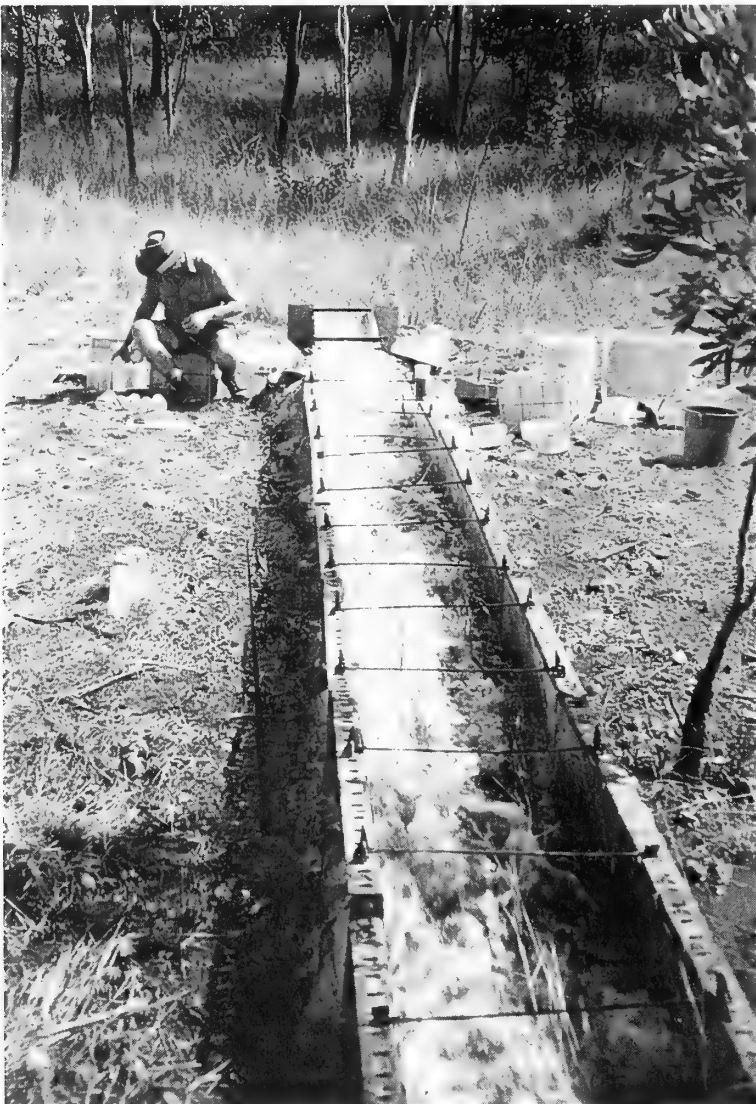
Figure 3b. A concentrated flow simulation experiment, in which the discharge of water through the race, sealed to the surface, provides data on the processes of erosion of the surface under controlled hydraulic conditions.
