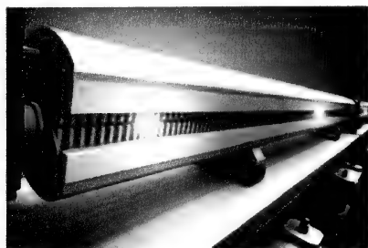
Figure 18: The LCLS undulator is made up of thousands of permanent magnet wiggler magnets.
