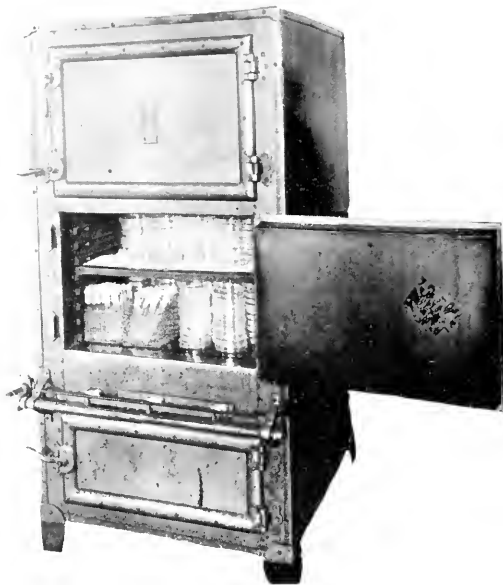
FIG. 2. HOTEL SIZE GAS OVEN USED FOR HOT AIR STERILIZER
