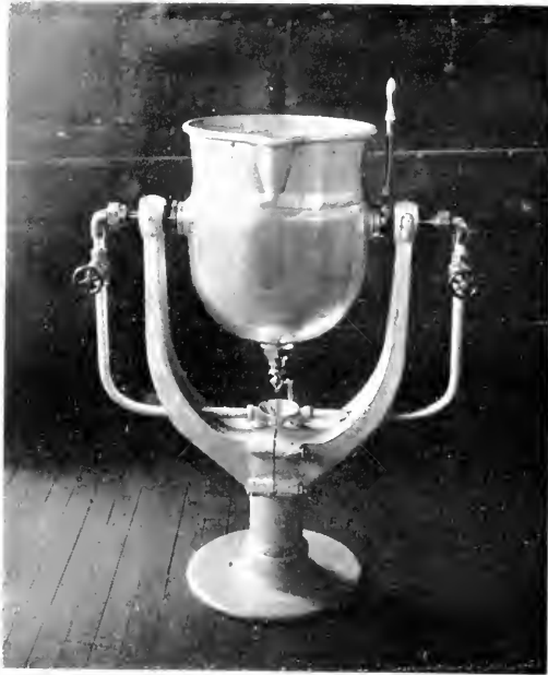
FIG. 1. STEAM JACKETED TRUNNION KETTLE USED FOR COOKING THE MEDIA
