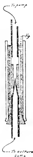
FIG. 2. SHOWING DETAILS OF THE CONNECTION BETWEEN THE CULTURE BOTTLE AND THE MERCURY PUMP
