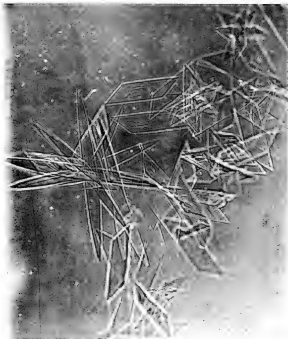
FIG. 12. The disodium salt of the acetyl derivative separated from a sodium chloride solution.
