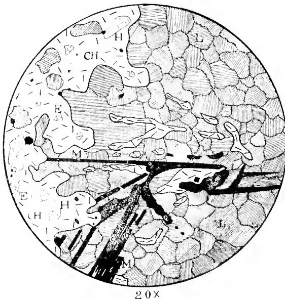
Fig. 2.—Contact of diorite-porphyrite with limestone in the Kamaishi Mine. H, Hornblende. E, Epidote. CH, Chlorite. L, Limestone. M, Magnetite.
