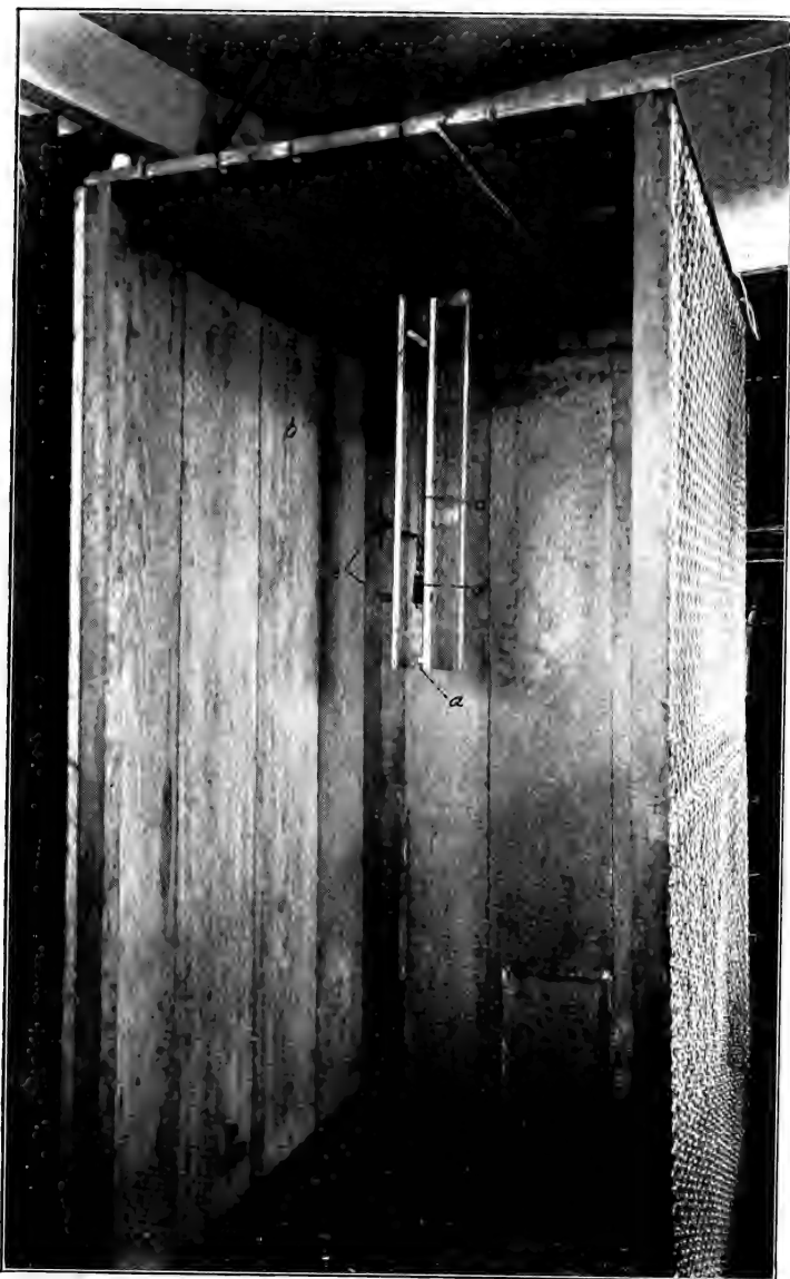
FIG. 3. New cage showing chute, a , with one side open; b , trap door; c , string; d , wire spring handle; e , rungs. Page 358.
