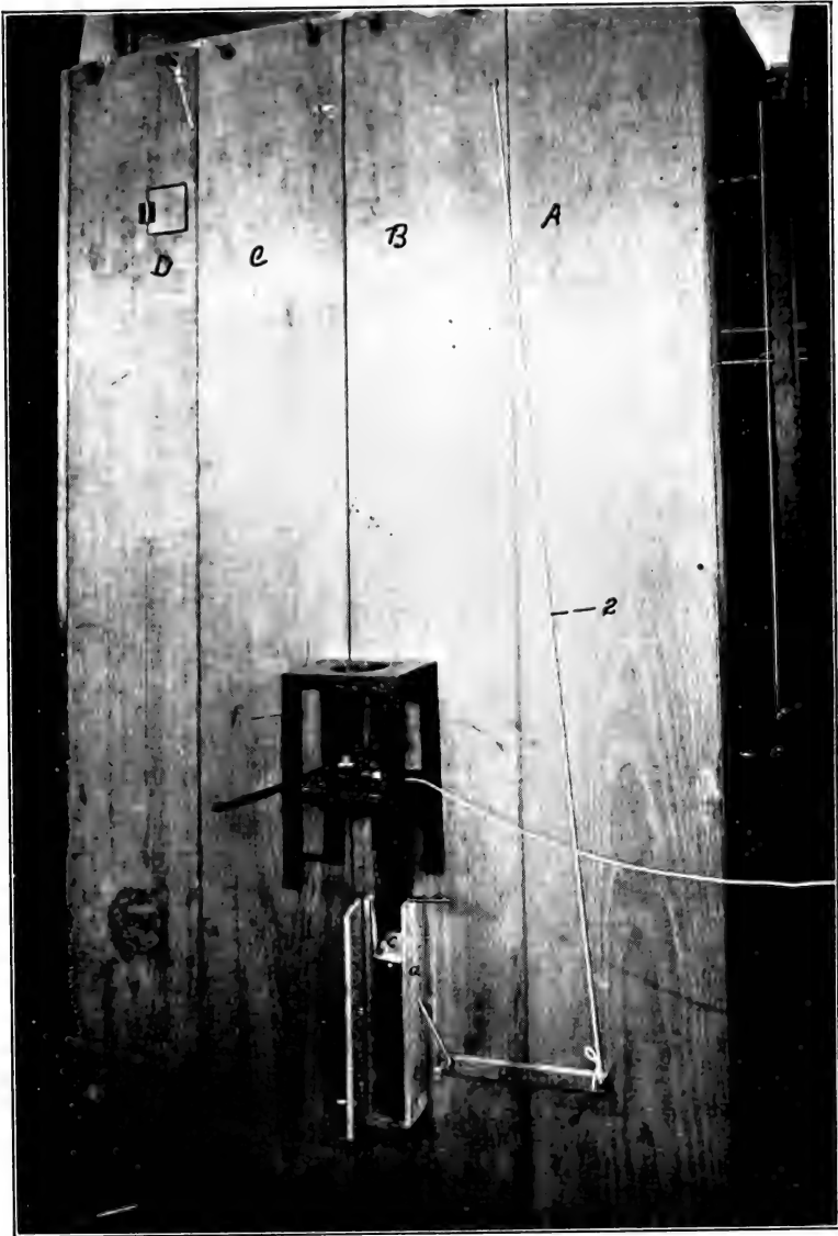
FIG. 12. New cage adjusted for the String Experiment; a , chute; b , bottom of chute on a level with opening into the cage; c , trap door; d , lever; 2, string 2; f , feeder. Page 426.
