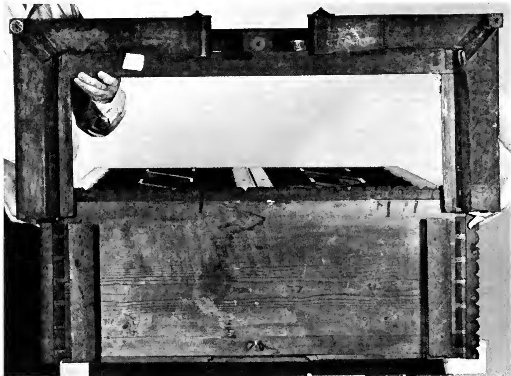
Figure 23. Detail showing the construction of the top and pediment of the bookcase section of the desk-and-bookcase illustrated in Figure 1.
