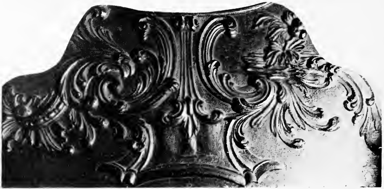
Figure 16b. A portion of a mahogany casting pattern, 1770-1785, possibly for a fireback, said to have been used at Durham Furnace in Pennsylvania; this pattern is attributed to the same carver who executed the pattern for Fig. 16. MRF S-12068.
