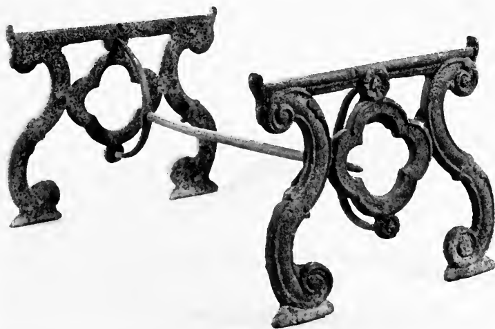
Figure 20. A stove base attributed to Marlboro Furnace, 1768-1790. HOA 14 \frac{1}{8} , DOA 17 \frac{1}{4} , LOA 28 \frac{3}{4} . The size of this base is appropriate for a stove the size of that represented by the plates in Figs. 16, 17, and 18. MRF S-11049.
