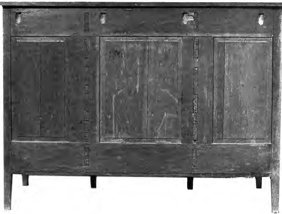
12a. Back view of sideboard in figure 12, showing the use of raised panels.
