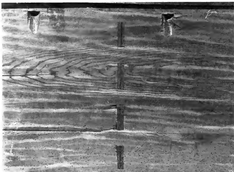
8a. Detail showing Lamond's use of vertical wedges to tighten mortised joints on the sideboard in figure 8.
