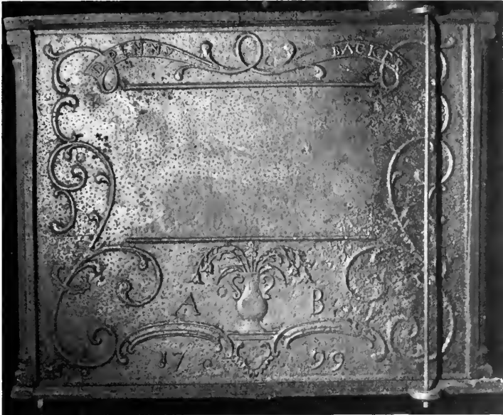
Figure 15. Side view of a six-plate stove run at the Redwell works for Derick Pennybacker while the furnace was under lease to Richard Patton. The overall dimensions of the stove body are: DOA 16", W'OA 27", HOA 33½". Courtesy Mauck's Meeting House. Photograph by the author.
