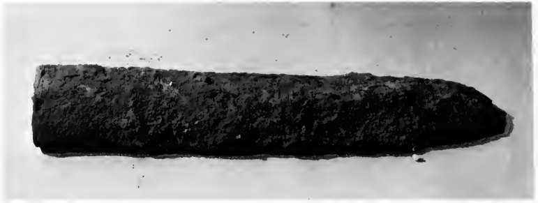
Figure 5. Fragment of a cast iron pig excavated at the Redwell Furnace site. LOA 16". Photograph by the author.
