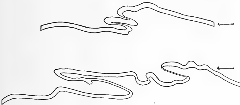
FIGS. 13 and 14.—Récurrent folds simulating nappes de recouvrement. These are overfolds whose lower limbs have been drawn out thin. Compare with Hobbs' contention that in overfolds the upper limbs should be thinned.
