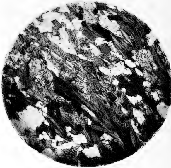
FIG. 6.—Biotite gneiss. (Magnification about 30 diameters. Ordinary light.) The photograph shows a great abundance of biotite (dark) and a complete absence of garnet due to the completion of the alteration. A single elongated prism of sillimanite occurs in the center of the field. Along the cleavages it is altered to chlorite (dark). The rectangular outline at the end of the prism is a basal section of sillimanite altered to chlorite.
