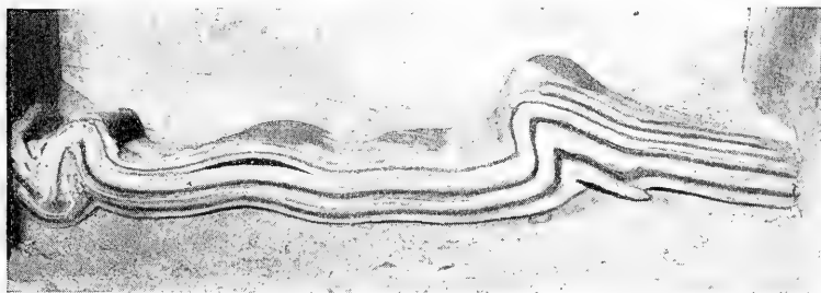
FIG. 6.—Original length 22 inches; compressed 4\frac{1}{2} inches. Layers 1, 3, 5, 7, 9 and 11 were 1 paraffin, 1 vaseline. Layers 2, 6 and 10 were 1 par., 2 vas. Layers 4 and 8 were 3 par., \frac{1}{2} vas., 1 plaster. Cavity developed under gentlest of the three anticlines. Folds developed first near the two extremities with less deformation in the middle portion. Pressure from the right.
