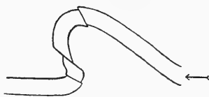
FIG. 17.—Break thrusts on stretched lower limb of anticline. The higher up on the fold, the steeper the angle of fracture. Thrust near crest has angle of 57^\circ .
