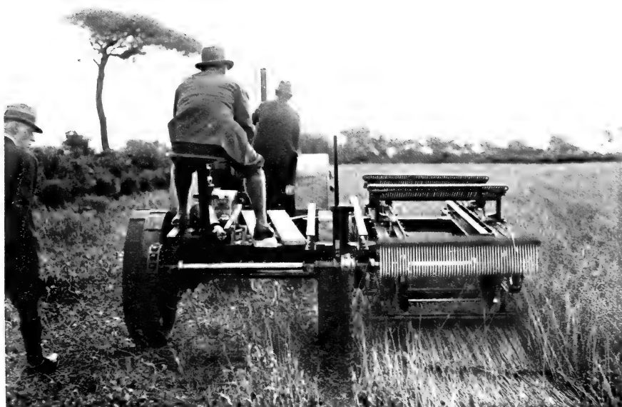
FIG. 2.—The Fibre Corporation Flax Pulling Machine.
