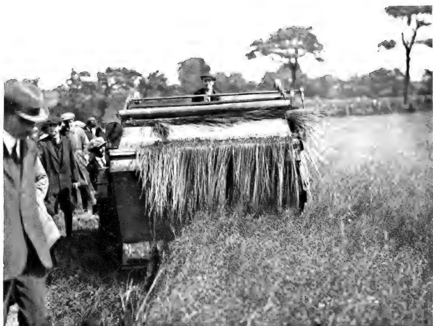
FIG. 1.—The Crawford-Bennett Flax Pulling Machine.
