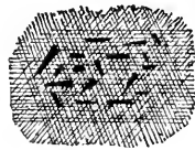
FIG. 5.—Cuneiform crystals in ruby and sapphire (enlarged 200 diameters).
