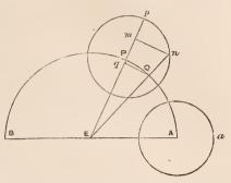
to EA; in other words,  $\angle p P n = \angle P E A = \theta$ . The point Q, in which En cuts the circle APB, is the true position of the planet; and PQ is the correction sought.
