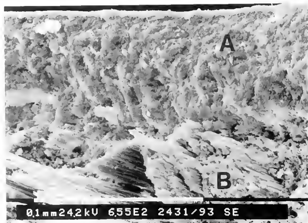
Figure 3. Electron micrograph of fracture along the shell height axis of A. balloti A = microcrystalline, calcitic outer layer; B = crossed-lamellar, calcitic middle layer.
