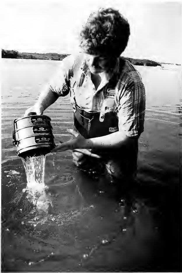
Figure 5. Sieving under field conditions. The use of 5.6-, 2.8-, and 1.0-mm sieves (top to bottom) in the Mohawk River (Crescent, NY) to collect zebra mussels, respectively, >11, 6–11, and <6 mm long.
