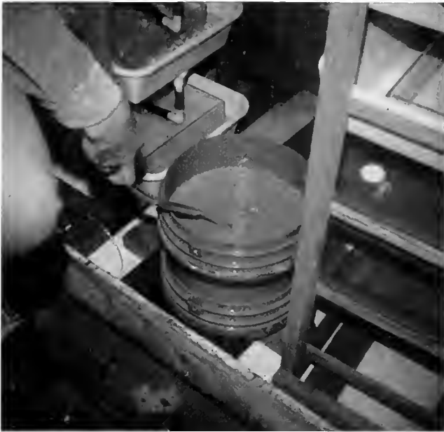
Figure 9. Inexpensive sieves were made from 5 gallon (19 liter) plastic buckets with tight fitting lids. Connector rings, (12" high) from the buckets ensured that no larvae were lost in the sieving process. Cascading glass "shelving" trays, (12" x 10" x 2") with attached mesh inside plastic "kitty litter trays" (15" x 12" x 3"), constructed for postset juveniles.
