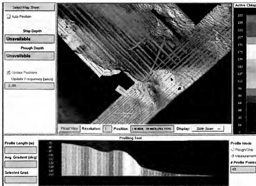
Figure 6. 2-D component of pipeline and cable-route planning tool. Multibeam sonar imagery is draped over bathymetry providing simultaneous depth and seafloor property information for route planner—prospective routes can be interactively explored with cross sections, gradients, and segment lengths displayed. The example above is from an application where real-time navigational information allowed the progress of the cable-laying vessel and the plow (cross hairs) to be monitored within the context of previously collected multibeam sonar data.
