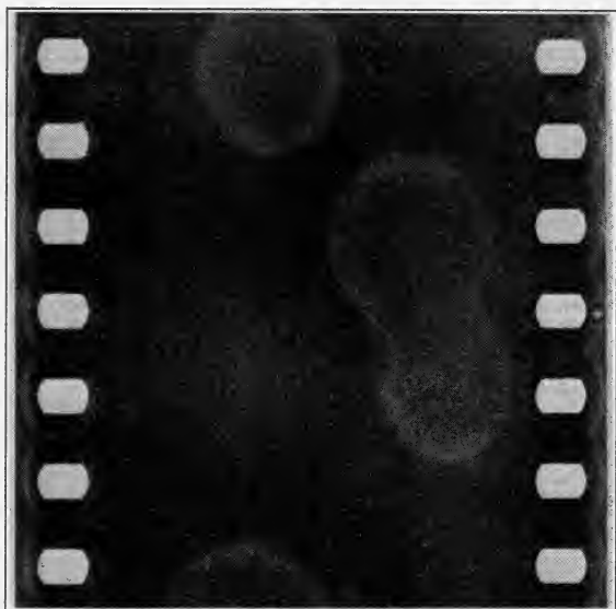
FIG 2. Appearance of scum on motion picture film after evaporation of drops of water containing dissolved salts.
