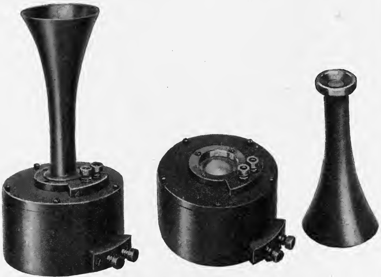
FIG. 1. An experimental loud speaker designed for high-frequency reproduction.
