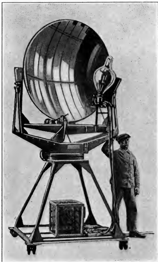
FIG. 8. A large mirror projector 1\frac{1}{2} meters in diameter, using a 10 kilowatt incandescent lamp.
