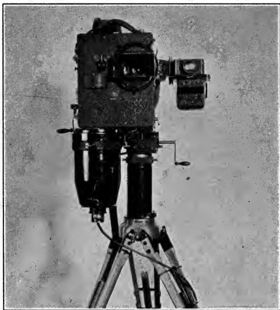
FIG. 1. 65 mm. camera mounted on tripod for location use, showing motor, housing and finder.
