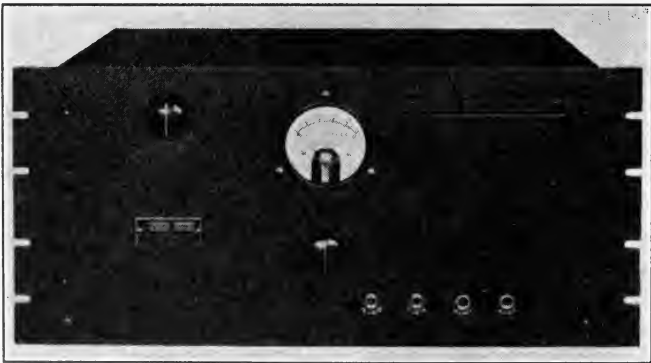
FIG. 12. Complete control unit designed for rack mounting.
