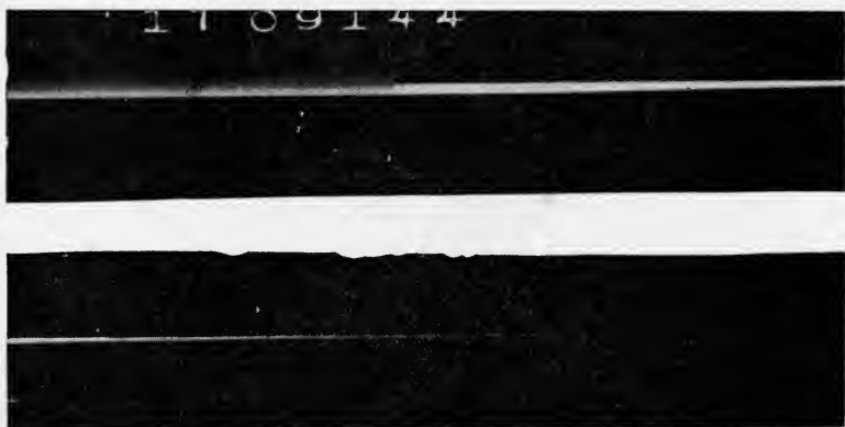
FIG. 4. Sound track obtained when the masking action after the cessation of modulation is too slow.
