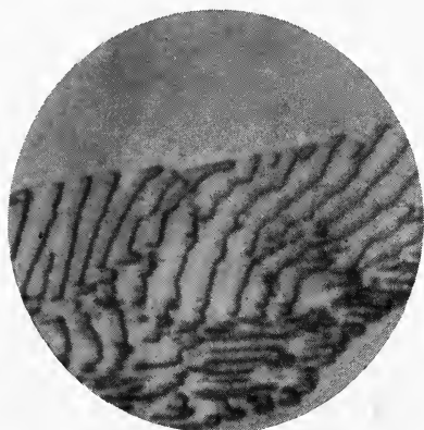
FIG. 1. Empty magnification. As can be seen from this picture, an increase in magnification is useless if accompanied by a decrease in the resolving power of the microscope.
