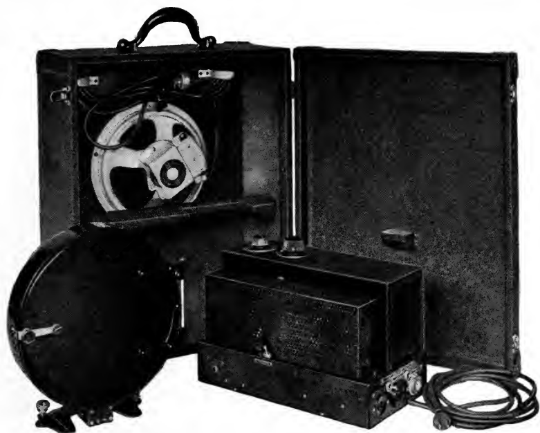
FIG. 5. Amplifier, loud speaker, cable, and upper magazine; the loud speaker operates through an opening in the front of the case (Fig. 1), the front of the case acting as baffle.
