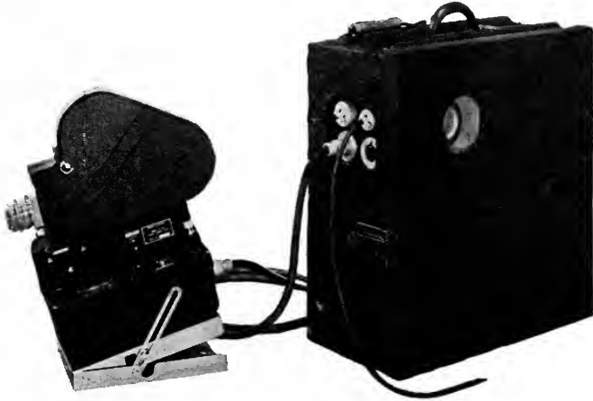
FIG. 12. Timing system, attached to Eastman high-speed camera ( Western Electric Co. and Eastman Kodak Co. ).
