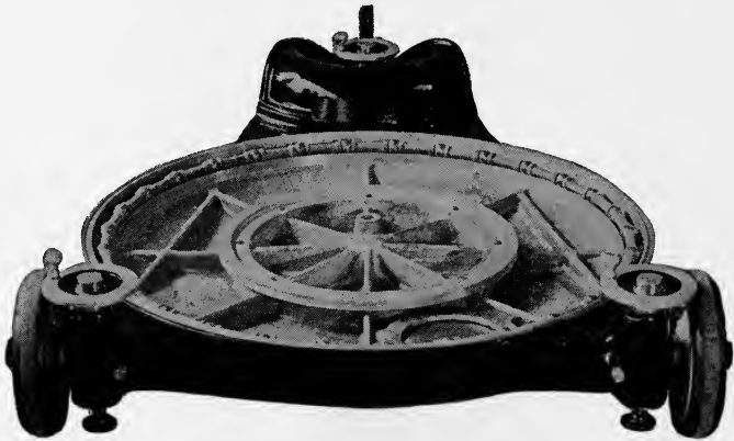
FIG. 3. The base, showing the large pulley for the panning drive and the large ball race.
