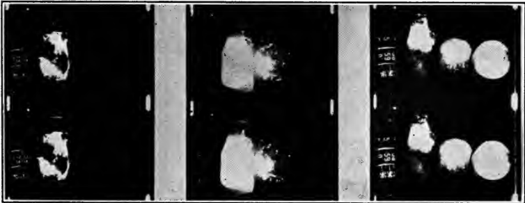
FIG. 13. Records made with Eastman high-speed camera and Western Electric timer: ignition of Mazda photoflash lamp connected to electric circuit, which in turn ignites successively two other lamps with their glass surfaces in contact. Total time interval 0.16 sec. ( Western Electric Co. ).
