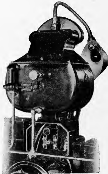
FIG. 4. Close-up of rear of rheostat unit, showing rheostat handle interlocked with the water supply, and motor reversing switch on the starting handle.
