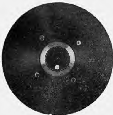
FIG. 9. One of the pole-pieces, showing the metal plate shellacked to it.
