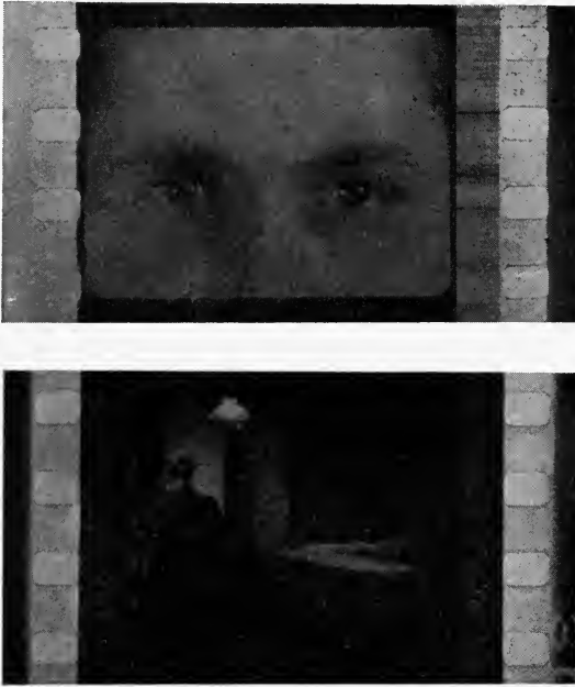
FIG. 1. Illustrating a wide difference in the density of sound-tracks in two scenes of a single production.
