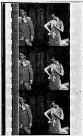
FIG. 1. Variable-density sound-track on film.
