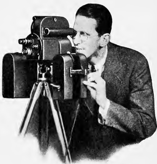
FIG. 10. Sixteen-mm. sound camera equipment set up on tripod.
