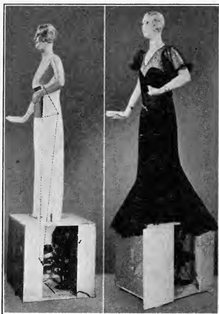
FIG. 4. Continuous display apparatus, exhibited at the Century of Progress Exposition, 1934, at Chicago; the mirrors and path of the light rays are shown in the left-hand view.
