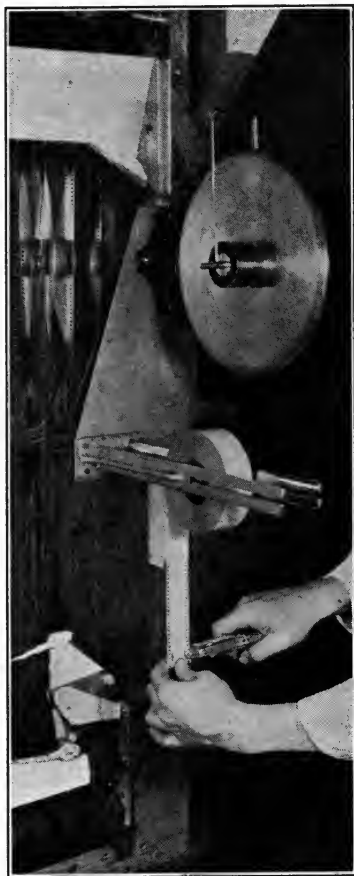
FIG. 4. View of the demountable feed stock and rewind as used in threading the rack.
