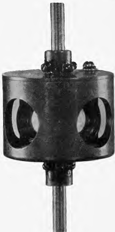
FIG. 4. Early model of four-way lens in mounting.
