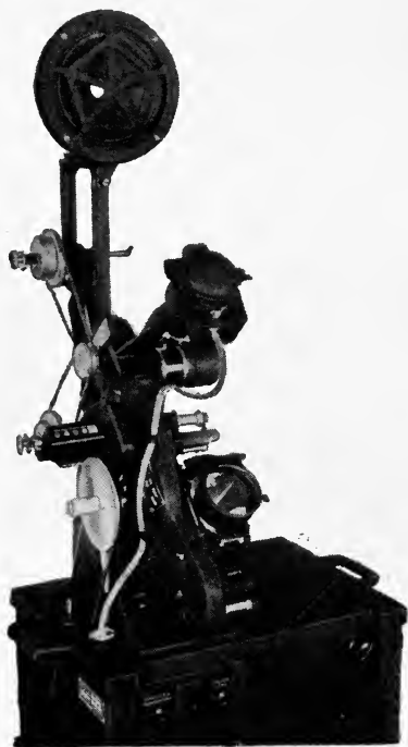
FIG. 7. Film viewing and sound reproducing machine, model UDC .
