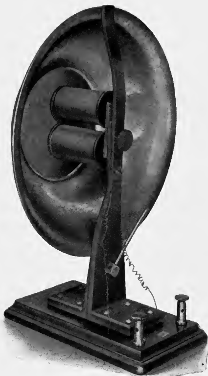
FIG. 3. Direct radiator, invented by Gray.
