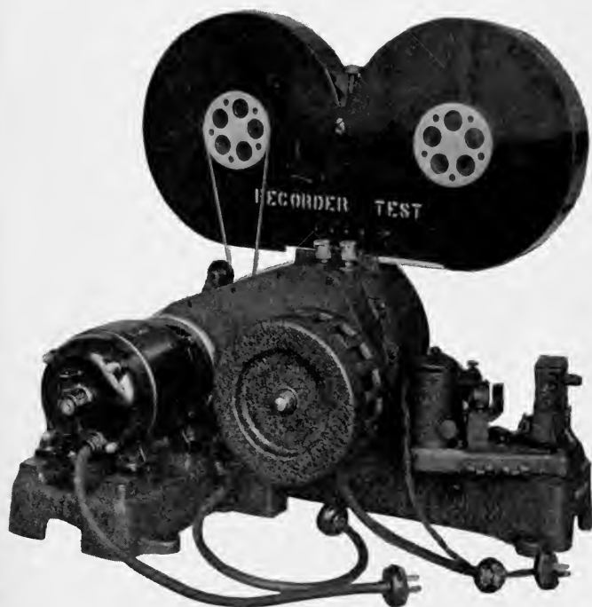
FIG. 11. Type PR-4 recorder, showing flywheel and driving magnet.
