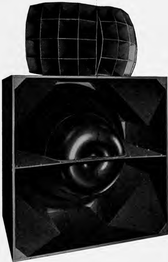
FIG. 9. Experimental 2-way horn system.
