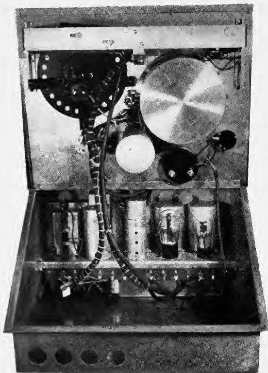
FIG. 2. Interior of densitometer, showing arrangement of motor disk, and illuminating lamp.
