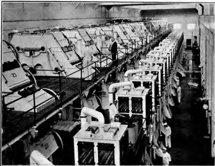
FIG. 3. Roll coating machines, in which the dope is cast upon large wheels for the preparation of film support.
