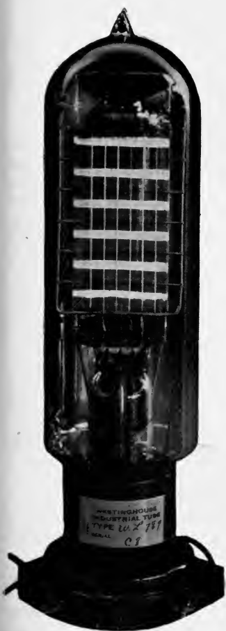
FIG. 1. The effect of the electrons striking the plate, which is coated with willamite, is seen in luminous bands. The width of these light bands may be varied by changing the voltage of the grid or the plate.
