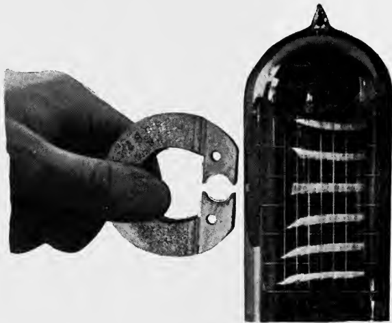
FIG. 4. Showing the magnetic effect upon the fluorescent pattern.
