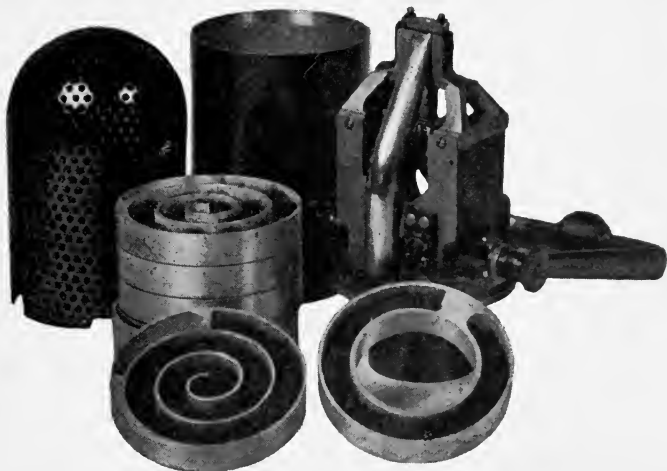
FIG. 3. Unidirectional microphone, disassembled.
