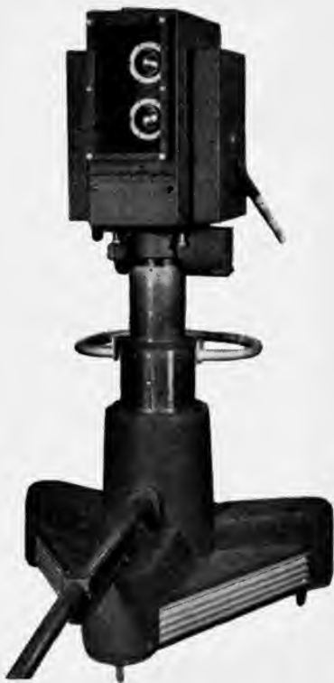
FIG. 19. A typical studio pick-up camera employing the Iconoscope.
