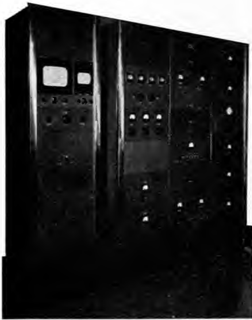
FIG. 6. Electrical equipment of the telecine channel.
