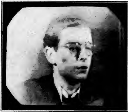
FIG. 6. Photograph made on a receiver 20 miles from the transmitter. No make-up used; camera exposure, 10 sec.
