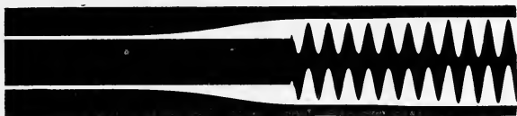
FIG. 2. Enlargement of sound-track.
