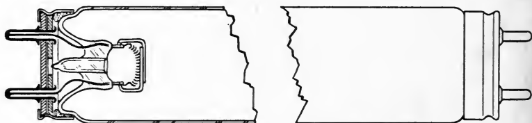
FIG. 1. Internal construction of a fluorescent lamp.
