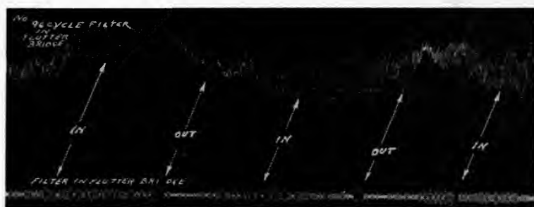
FIG. 9. Variations in 96-cycle frequency modulation with negative and print sprocket-holes passing in and out of register.
