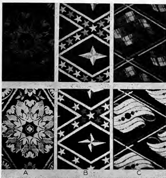
FIG. 11. Fluorescent carpet patterns, shown as illuminated with ( top row ) visible light and ( bottom row ) black light. Pattern B has approximately 50 per cent more brightness than A or C .
