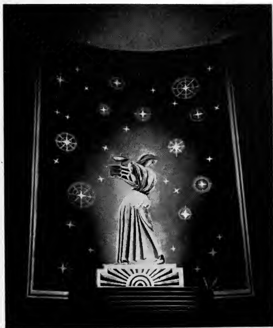
FIG. 4. Fluorescent mural over exit door at front of auditorium. Black-light unit below mural in architectural element over door.
