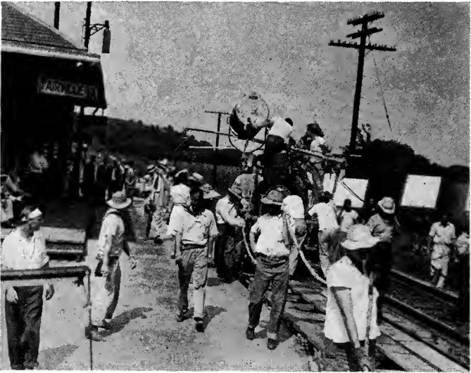
Dolly shot on location, with booster lights. Dolly tracks alongside rails permit trucking shot of incoming train. ( Paramount Pictures. )
