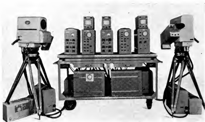
FIG. 1. Dual camera chain equipment.
