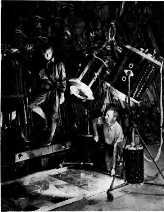
Effect of water reflections, produced by moving broken glass reflecting light from shots.
