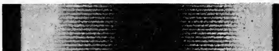
FIG. 2. Photomicrograph of 7000-cycle track printed on Eastman 5301 stock, using white light coated lenses and white light exposure. Print Density 1.2; Print Gamma 2.0.
