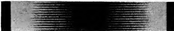
FIG. 5. Photomicrograph of 7000-cycle track printed on Eastman 5302 stock, using white light coated lenses and white light exposure. Print Density 1.2; Print Gamma 2.5.
