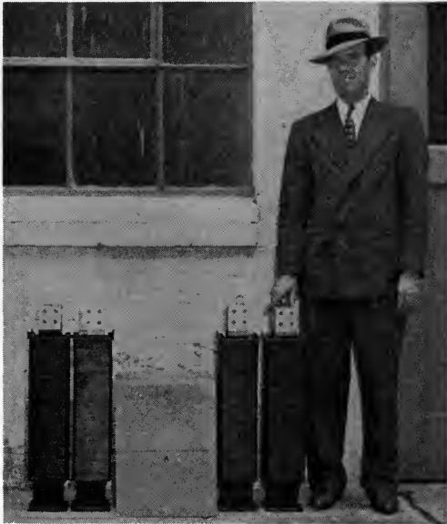
FIG. 3. The new-type filtering equipment used on a set requiring 5000 amperes.
