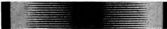
FIG. 6. Photomicrograph of 7000-cycle track printed on Eastman 5302 stock, using ultraviolet coated lenses and ultraviolet exposure. Print Density 1.2; Print Gamma 2.5.
