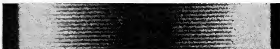
FIG. 1. Photomicrograph of 7000-cycle track printed on Eastman 5302 stock, using white light uncoated lenses and white light exposure. Print Density 1.0; Print Gamma 2.0.
