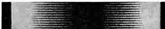
FIG. 3. Photomicrograph of 7000-cycle track printed on Eastman 5301 stock, using white light coated lenses and ultraviolet exposure. Print Density 1.2; Print Gamma 2.0.
