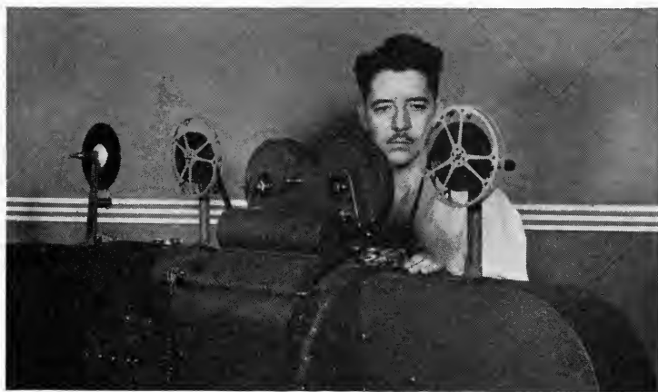
FIG. 3. The testometer, used for checking timing. The left side contains a time-scale sensuometer.
