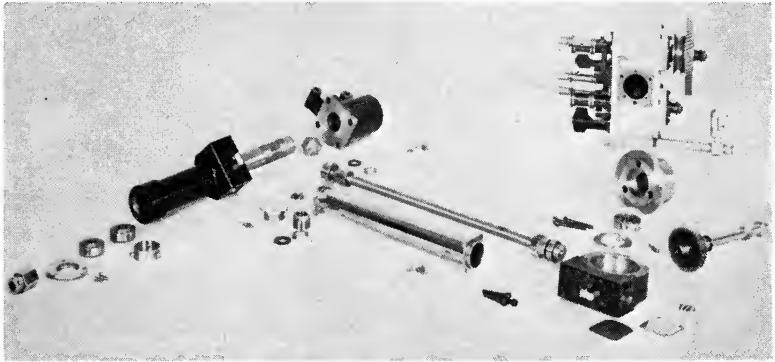
FIG. 4. Disassembled view of shutter-shaft driving system for General Electric television projector.
