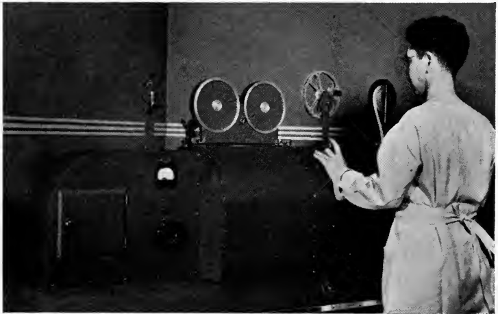
FIG. 4. Using the testometer as a sensitometer.
