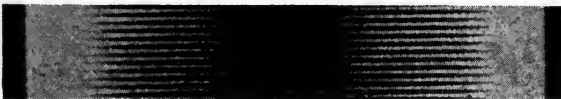
FIG. 4. Photomicrograph of 7000-cycle track printed on Eastman 5301 stock, using ultraviolet coated lenses and ultraviolet exposure. Print Density 1.2; Print Gamma 2.0.
