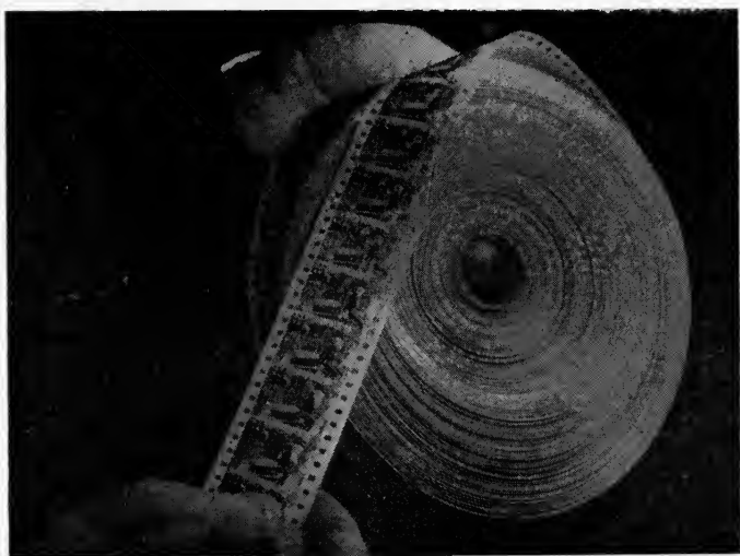
FIG. 2. A close-up of a roll of motion pictures on a paper ribbon.
