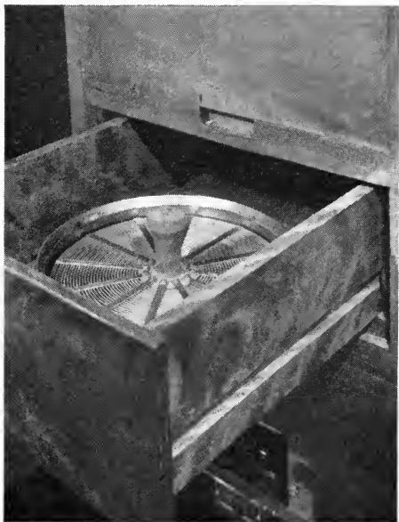
FIG. 6. Open drawer of drier showing processing reel in place.
