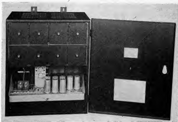
FIG. 23. Low-voltage power supply, MI-10505 .
