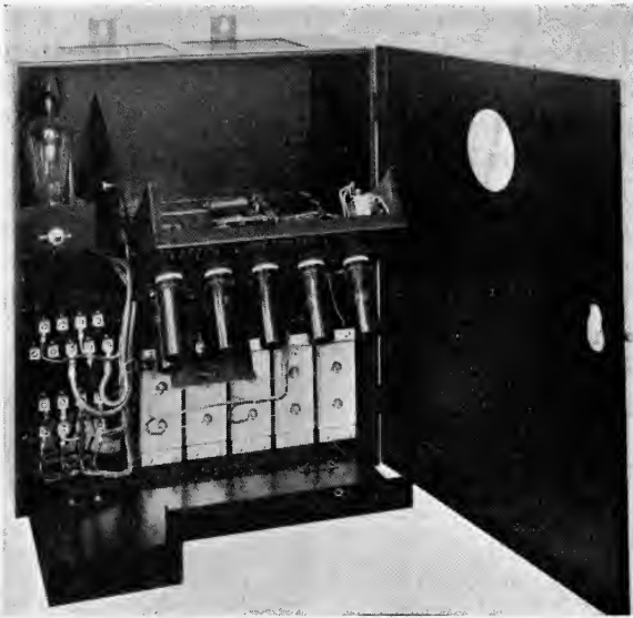
FIG. 20. Plate supply with units exposed for servicing.
