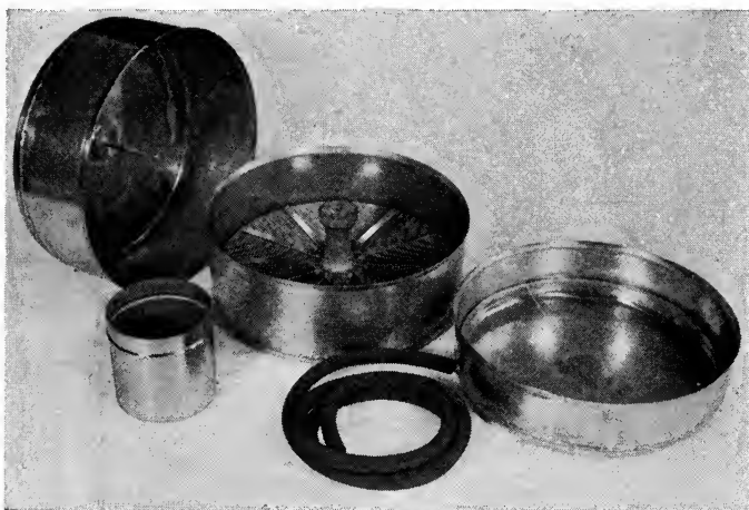
FIG. 3. The processing and washing tanks with a reel in position. Temperature control tank in foreground.
