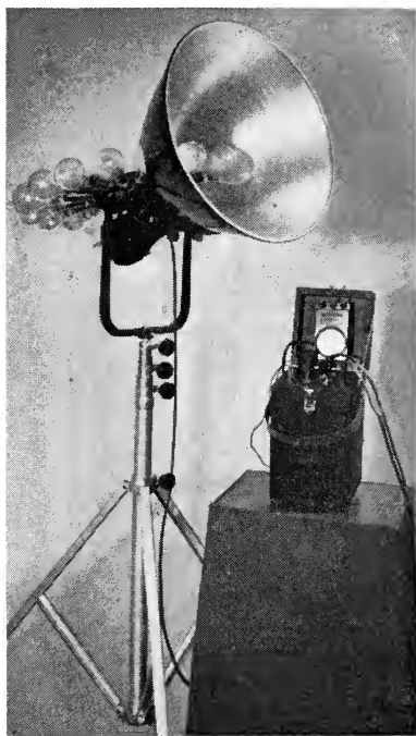
FIG. 7. Continuous flash lighting unit with "power patch" and control boxes.
