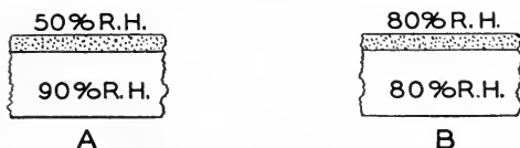
FIG. 4. Effect of drying time on moisture distribution in motion picture positive film: A —Relative humidity with which each layer is in equilibrium at end of drying period; B —Relative humidity with which each layer is in equilibrium after standing in roll form.
