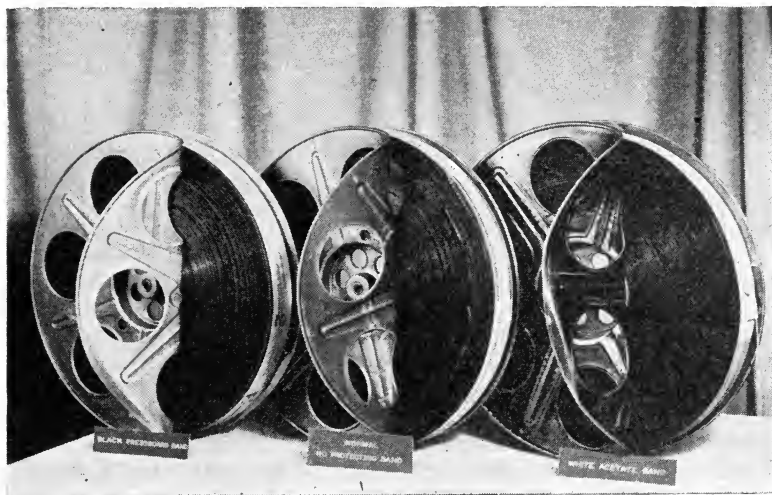
FIG. 13. Comparative edge condition of film protected by stiff bands (not shown in picture) with edge condition of film wrapped with customary paper band.
