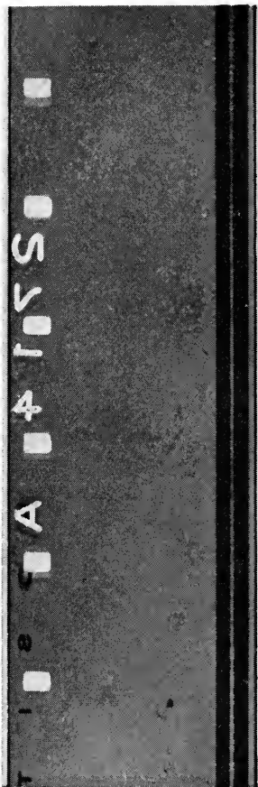
FIG. 3. A 16-mm sound track as it may appear if the recording is done on "A Winding" stock.
