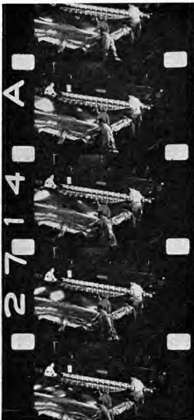
FIG. 2. Original 16-mm photography with edge numbering as it will appear when marked with the numbering head described in the text.
