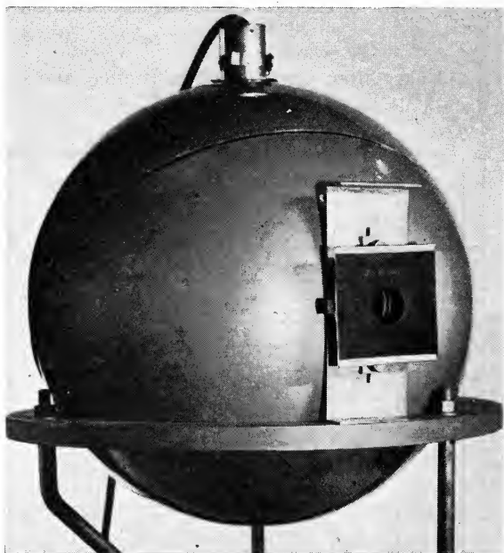
FIG. 5. Integrating sphere with a calibrating stop mounted over sphere opening.
