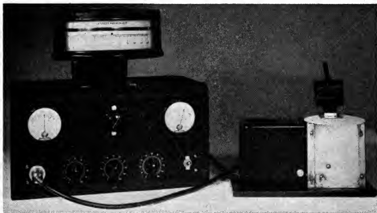
FIG. 4. Instrument for photoelectric examination of dirt traces.
