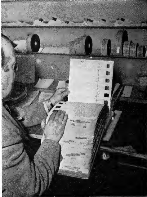
FIG. 2. The catalogue pages contain 7 frame apertures in which the film frames are placed for viewing.
