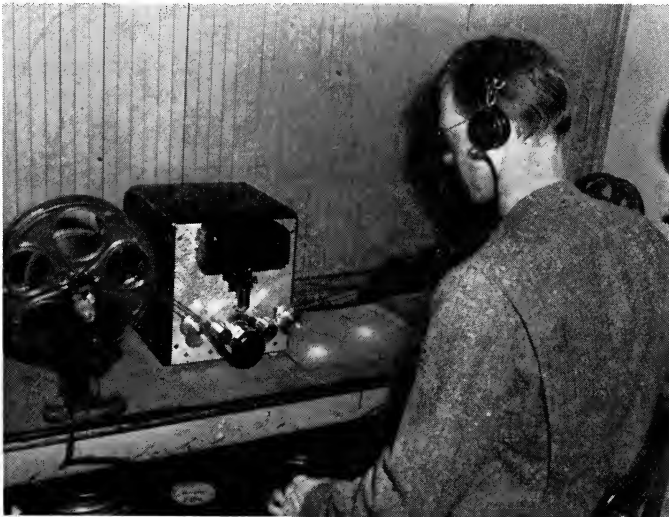
FIG. 1. Film noise spotter developed by Twentieth Century-Fox Studios.
