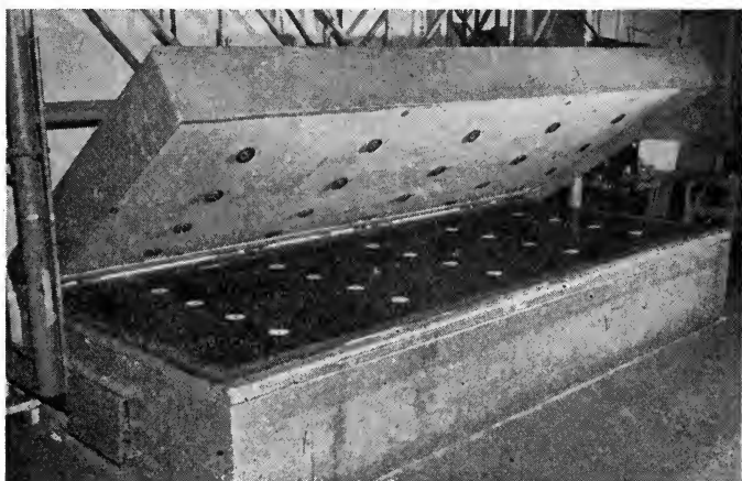
FIG. 4. Consolidated Vultee's Downey plant designed and constructed this X-ray printer for both primary and after-glow exposure procedures. It will accommodate 4 × 12-ft sheets.
