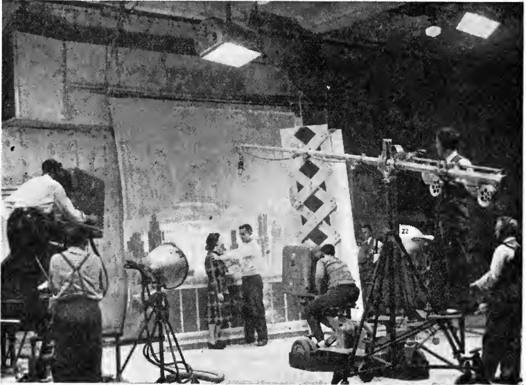
FIG. 6. A television studio (WRGB) employing water-cooled mercury lamps, for both overhead and floor lighting equipment. Each unit contains 3 lamps operating on a 3-phase circuit.
