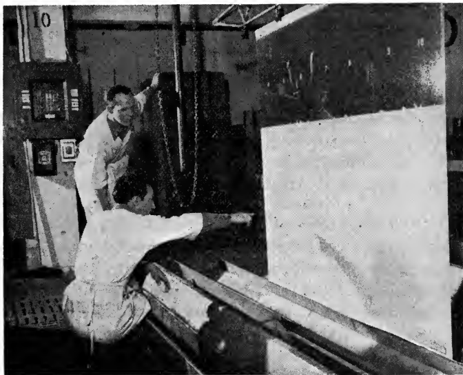
FIG. 3. Vertical tanks set in the floor are most efficient for processing large sheets of sensitized metal. A hoist is required for handling heavy pieces as shown in this installation at Consolidated Vultee Aircraft Corporation.
