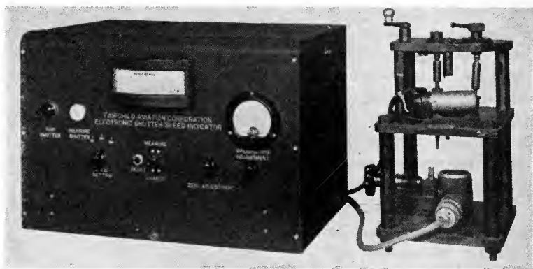
FIG. 16. Direct-indicating shutter tester, with fixture for phototube, light source, and shutter holder at the right.
