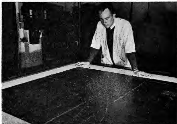
FIG. 8. Consolidated Vultee uses pin-located reflex negatives for the reproduction of large master drawings.
