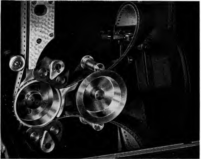
Fig. 9—Bipack side showing removable guide roller.
