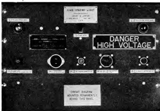
Fig. 6—Front of Cine-Strobe-Light power pack, showing switches, plugs, and pilot lights. All are marked to correspond with the circuit diagram; all are different in size and shape to prevent any possibility of misconnections.
