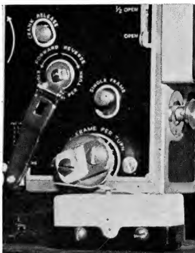
Fig. 3—Contactor built onto one-frame-per-turn shaft of camera, operates microswitch to close trigger circuit of flashtube.
