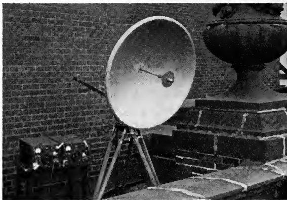
Fig. 4—1300-megacycle relay transmitting equipment at repeater station.
