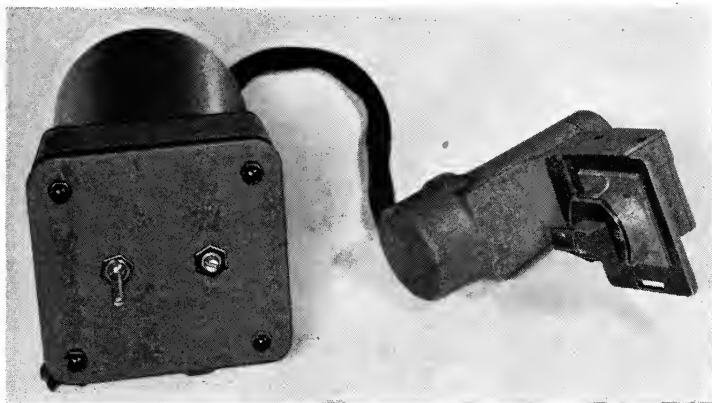
Fig. 14—Phototube monitoring optical system and transformer assembly.
