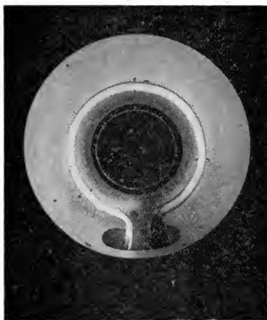
Fig. 4—Toroidal-parabolic reflector with FT-429 tube flashing. Note even reflection and light distribution.
