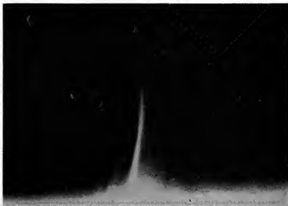
Fig. 5—A slight crease in the base allows local entrapment of a greater volume of developer which in turn develops more before fatigue with consequently greater density. Such a crease effect due to development is difficult to distinguish from pressure fog. The above vertical arc corresponds with the crease.
