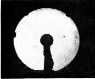
Fig. 5. Image of the Light-Collecting Mirror of a Typical Suprex Carbon Arc Lamp; formed by the motion picture projection lens in a plane close to the front surface of this lens.
