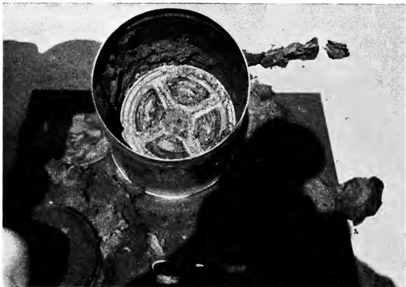
Fig. 2. Reel of film which had spontaneously ignited during a test at the National Bureau of Standards.
