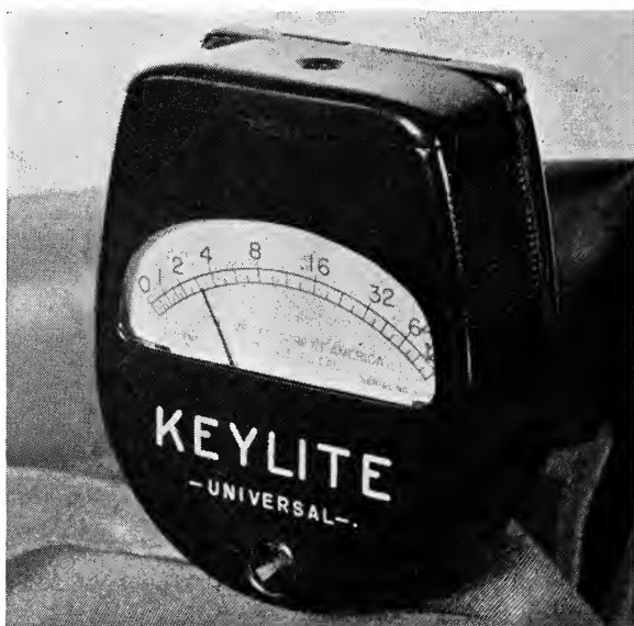
Fig. 6. Exposure meter designed to measure the key-light.
