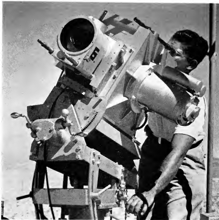
Fig. 3. The Bowen Ribbon Frame Camera can be accurately aligned to photograph an expected rocket or missile trajectory. The camera operates at from 30 to 180 frames per second, recording on 5\frac{1}{2} -in. aerial roll film.
