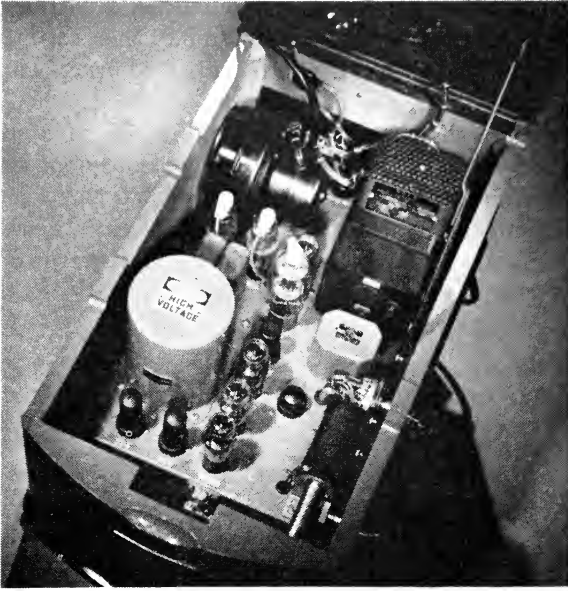
Fig. 14—Instrument chassis—showing high-voltage transformer, control and rectifier tubes, lamp-voltage stabilizer, and zero-adjustment solenoid.
