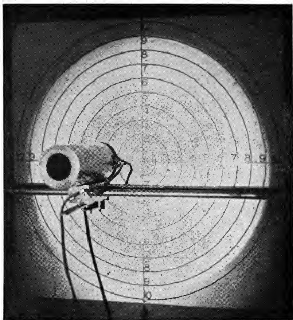
Fig. 8. Crater Image Board; adapted for tracing the red, green, and blue intensity distributions across the crater.
