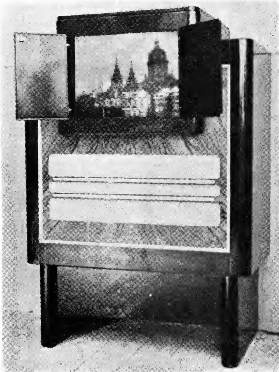
Fig. 10. Model of a home cinema fitted with a special projector (mounted in the cabinet) for cellophane film. The projected picture satisfies high requirements regarding sharpness as well as gradation.
