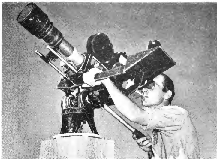
Fig. 5. Mitchell Chronograph 35-mm Tracking Camera with 18-in. lens used at Naval Ordnance Test Station to determine missile attitude, roll, and separation information.
