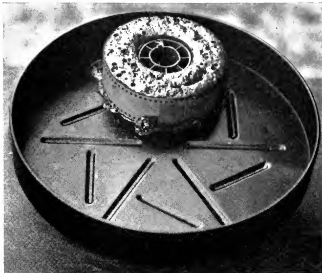
Fig. 5. Sample of film in the fourth stage of decomposition.
