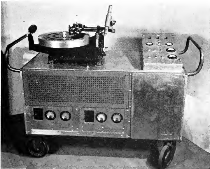
Fig. 3. Recording and reproducing equipment and controls, with all electronic equipment mounted in portable cabinet.
