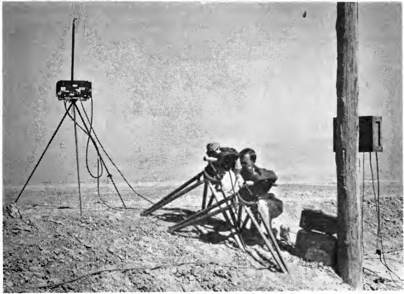
Fig. 8. Two 16-mm Eastman High Speed Cameras are aligned to cover the launching of a guided missile. The radio receiver at left receives a broadcast 1000-cycle note and transmits it to timing lamps in the cameras.
