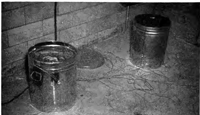
Fig. 1. Container in which reel of film was placed, showing thermocouple wires.
