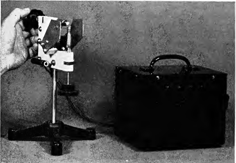
Fig. 15. Experimental 1-kw a-c open-air concentrated-arc lamp and transformer unit.
