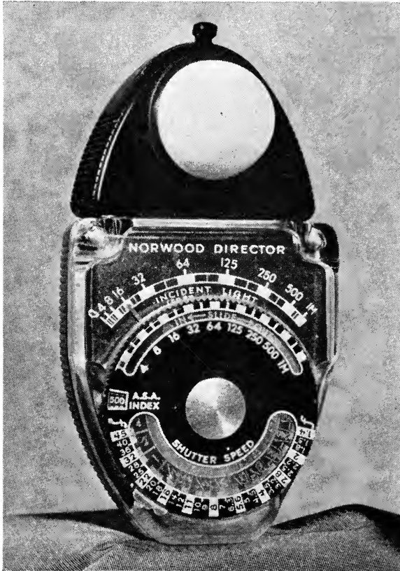
Fig. 4. Exposure meter designed around hemisphere light-collector.
