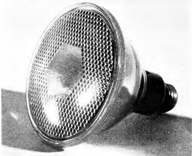
Fig. 3. PAR-38 Flood; 150-w, 1,000-hr life.
