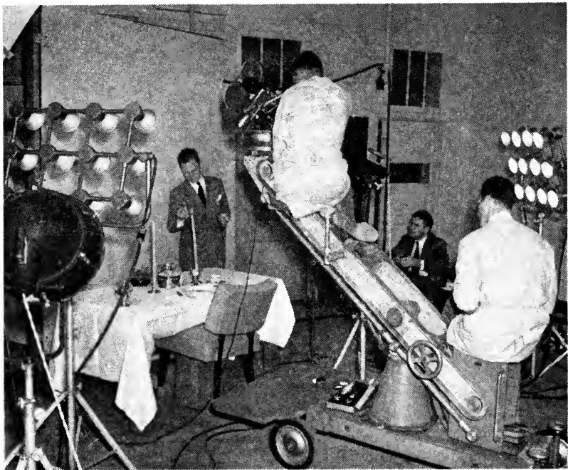
Fig. 7. Lamp banks assembled and ready for use in small studio scene.
