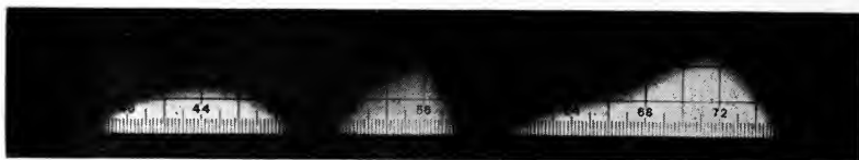
Fig. 4. Wedge spectrogram showing sensitivity peaks of magenta, yellow and cyan layers.
