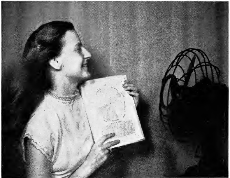
Fig. 4. Electric-flash infrared photograph; note "freezing" of fan blade.
