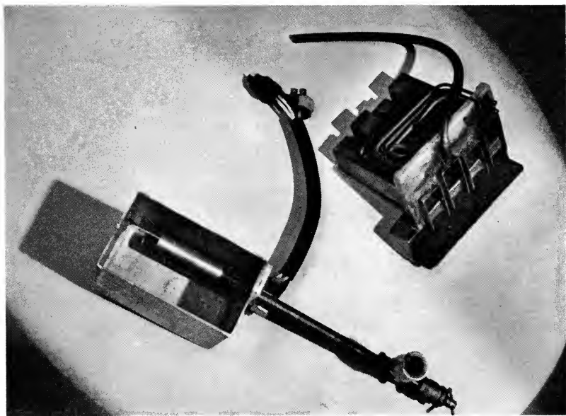
Fig. 2. Tank section for 16-mm rapid processing machine; heat-exchanger jacket at left, and four processing tanks with preheating coils at right.
