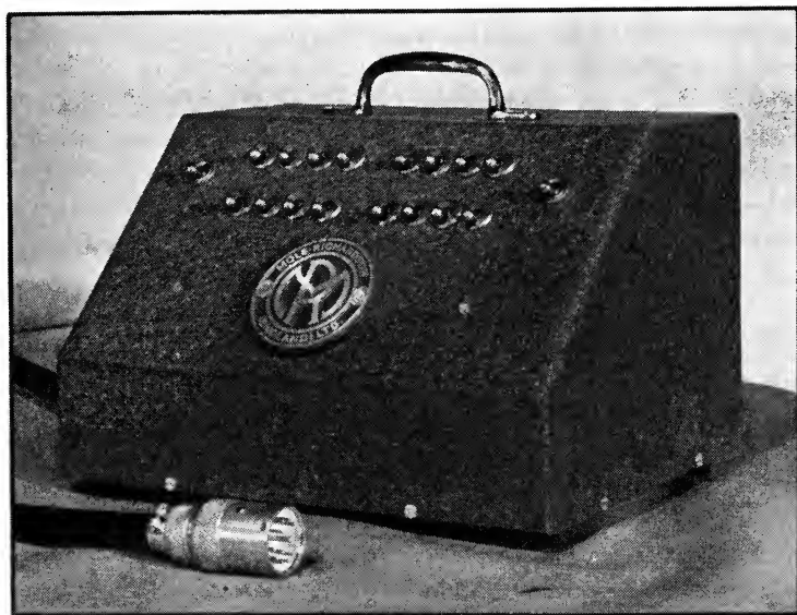
Fig. 7. Control box for lightning effects.
