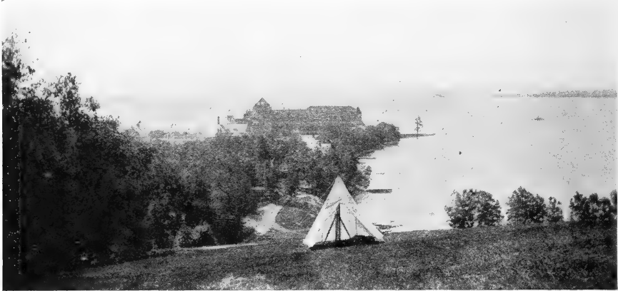
Fig. 6.—Magnetic observing tent and magnetic station at Kineo, Maine (Moosehead Lake), in 1910. Field observations are made within the tent to protect the instruments against wind, rain, or direct rays of the sun.
