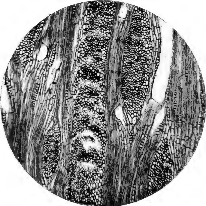
Grevillea robusta —Tangential section showing part of a large multiseriate ray in centre and right and left, cut transversely; fibres and wood parenchyma alternately in other parts, vessel in right top. \times 40 .
