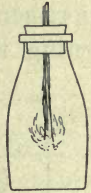
FIG. 17. — A lighted splinter burns for a time in the inclosed air of the bottle and then "goes out."
