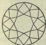
FIG. 100. — How a diamond is cut so as to give it many "facets," or surfaces, for the flashing of light.
