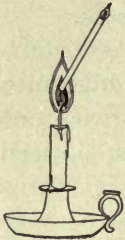
FIG. 20. — In the center of a candle flame there is a combustible gas that can be drawn off through the glass tube and burned.
