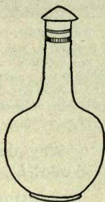
FIG. 45.— As water oozes through the porous jar, it evaporates and cools the water inside the jar.
