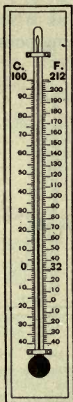
FIG. 42. — In the Centigrade thermometer the freezing point is called 0° C. and the boiling point 100° C.
