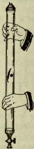
FIG. 64.— In a vacuum light bodies and heavy bodies fall at the same rate.
