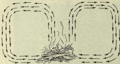
FIG. 52. — Air currents over a fire, or over the heated earth, rise to a certain height, then flow out horizontally, and finally fall again to the earth as they become cooled. Tell why.
