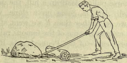
FIG. 196. — By using a crowbar with a support a man can lift a heavy stone from the ground.
