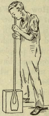
FIG. 179. — The lump of soft glass attached to the hollow tube is put into the mold. The workman, or a current of compressed air, blows into the glass lump until the glass has the shape of the mold.
