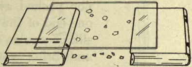
FIG. 136. — When the upper surface of the pane of glass is rubbed, it becomes charged, and objects under it are affected by the charge.
