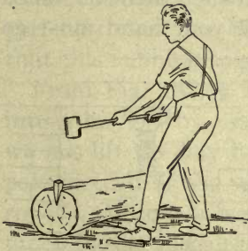
FIG. 210. — How a log may be split in two.
