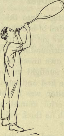
FIG. 178. — The glass blower blows a large lump of hot, softened glass into a hollow globe. When this is cut open, and then softened by heat, it forms a flat sheet.
