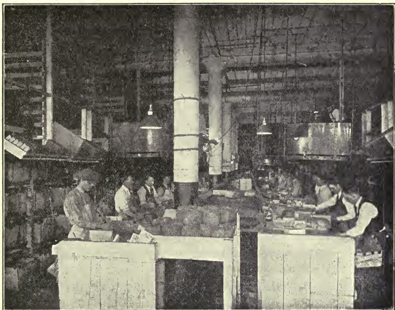
Fig. 167. A shipping room. After the packages are wrapped and addressed, they are conveyed by the moving belt, shown in the center of the picture, to the loading platforms.
