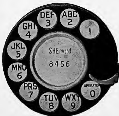
Fig. 73. The dial of a machine-switching telephone. The lettering on the dial varies in different localities.
