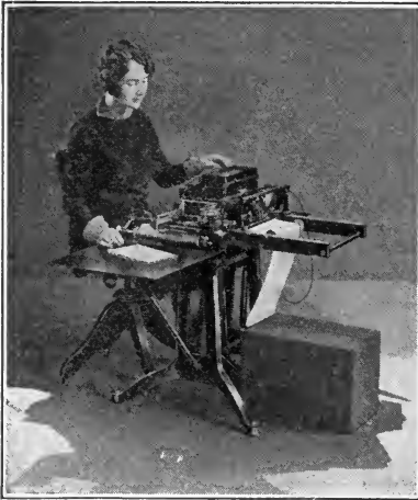
Fig. 160. The machines at which these young women are working will copy a purchase order (Fig. 159) and six duplicates in one operation.
