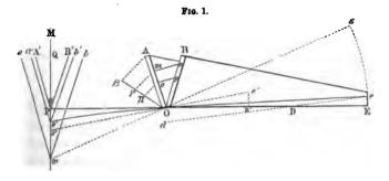
rough ground on their outer side, or covered with black varnish, may be of any size, but in general they should be from four or five to ten or twelve inches long; their greatest breadth being about an inch when the length is six inches, and increasing in proportion as the length increases. When these two plates are put together at an angle of 60°, or the
