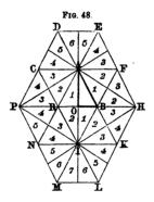
are equal. The field of view, represented in the figure by DEHLMP, is a truncated rhomb, consisting of no fewer than thirty-one images of the aperture AOB. The figure is composed of two hexagons DEFBEC, EBKLMN, every division of the hexagon consisting of two reflected images, and of two rhombs CENP, FBKH, each of which is composed of four reflected images.
