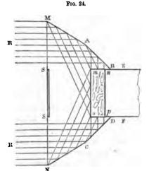
box. If the angle formed by the sides of the cone is such that a ray of the sun's light falling upon M, the upper margin of the reflecting surface of the cone, is reflected to o, the lower side of the object-box, then all the rays of a beam of
