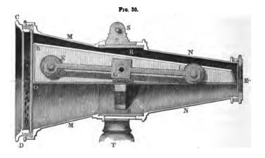
these reflectors, BOE, is fixed to the ring RR, by the intermediate piece KGL. The reflector is screwed to this piece by the adjustable screws K, L; and the piece KGL is again fixed to the ring RR, by two screws seen above and below G, in Fig. 31. Hence the tube, consisting of the cones MM, NN, and the ring RR, are immovably connected with the mirror BOE. The surface of the reflector BOE is adjusted by the screws at K and L, till it passes accurately
