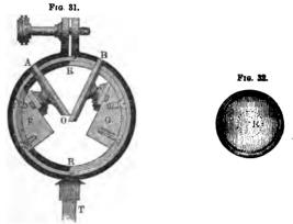
means of an intermediate piece, similar to KGL, the arm  $\mathbf{F}$  of which, corresponding to G, passes through an annular space or open arch, of more than 90°, cut out of the circumference of the inner ring RR. The arm  $\mathbf{F}$  is fixed to the outer ring rr by two screws, seen above and below  $\mathbf{F}$ ; and the reflector  $\mathbf{A}$  o is fixed to the bar corresponding to KL, Fig. 30, by similar screws, for the purpose of adjusting it.
