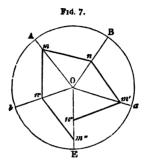
0 m = 0 m' = 0 m'', and 0 n = 0 n' = 0 n'', consequently since 0 m is by hypothesis greater than 0 n, we shall have 0 m'' greater than 0 n''; that is, the images m' n'', n' m'', will not coincide. As 0 n approaches to an equality with 0 m, 0 n'' approaches to an equality with 0 m'', and when 0 m = 0 n, we have 0 n'' = 0 m'', and at this limit the images are symmetri-
