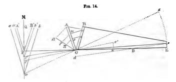
the eye is placed at s, the aperture A o B will be projected into a b  $\omega$  upon a plane passing through M N and at right angles to E O'; but the orthographic projection of A B O upon the same plane is A' B' O', or, what is the same thing, the reflecting surfaces of which A O, B O are sections, will, when prolonged, cut the plane passing through M N in the lines A' O', B' O'; hence, rays from the objects situated
