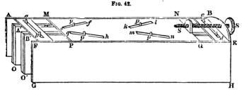
F H, of this frame, are kept together by four cross pieces, a b, c d, etc., the other two corresponding to these being invisible in the figure. The two reflectors, the ends of which are seen at A' 0, B' 0, are each fixed to a plate of metal p p, a section of which is seen in Fig. 44. Each plate of metal has four cylindrical pins, p, p, etc., both on its upper and under edge. The two pins nearest the ends
