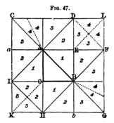
the mirror B o, and the other half a reflexion of half of B H b, from the mirror A o; and the triangle D E F consists of two half images, which are reflexions of the two half images in I O H. The remaining triangle D L F is a reflection of I K H, from the mirror A B, and is therefore formed by four reflexions.
