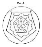
the radial line 10, o, then the images of all these objects will also be similarly situated with respect to the radial lines that separate the sectors, and will therefore form a whole perfectly symmetrical, whether the number of sectors is odd or even.
