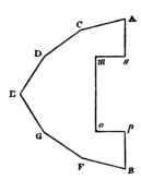
When the light is strong, a circular disk of fine grained white paper may be advantageously placed upon the outer face m o of the object-box.
